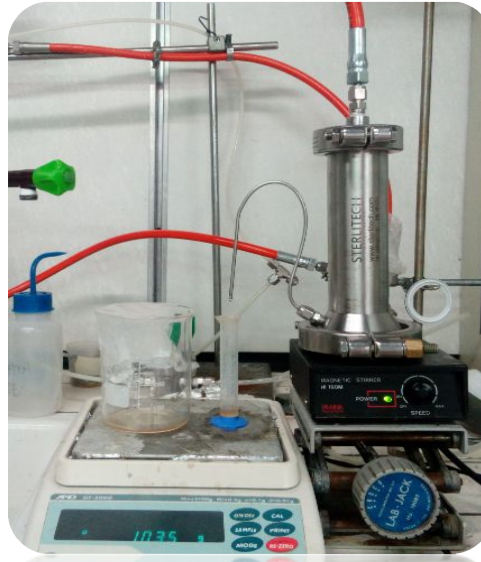
Figure 3. Stirred cell rig for microfiltration and nanofiltration membranes
