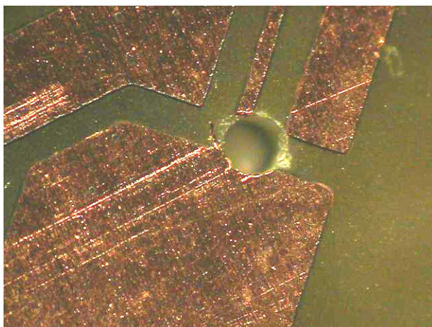
Fig. 36 Photograph of the micro-well with sensing electrode of 130um width
