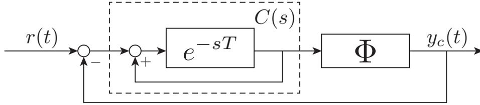
FIGURE 2.6: Continuous-time nonlinear RC scheme.
