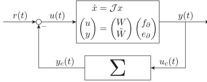
FIGURE 2.7: Feedback interconnection between a BCS in scattering form and the nonlinear system  $\Sigma$ .
