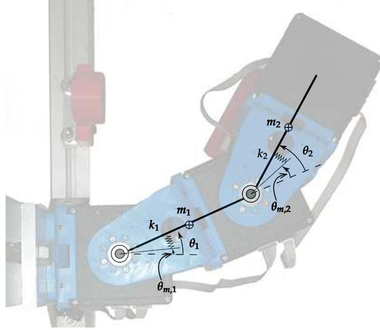
FIGURE 4.7: Two-link robotic arm with elastic joints based on QB-Move - Maker Pro VSAs.
