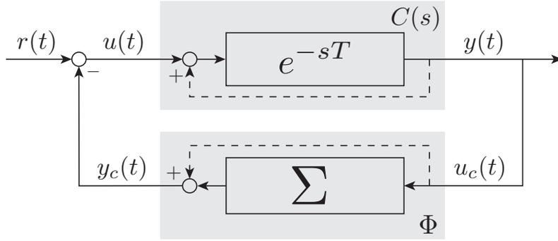
FIGURE 2.8: Equivalent representation of the RC scheme of Fig. 2.6.
