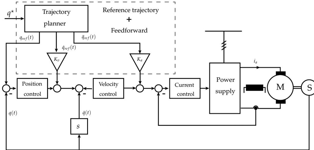
FIGURE 4.1: Standard cascade control structure with feedforward for electrical motor drives Leonhard, 2001.
