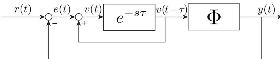
FIGURE 1.8: Continuous-time nonlinear RC scheme.
