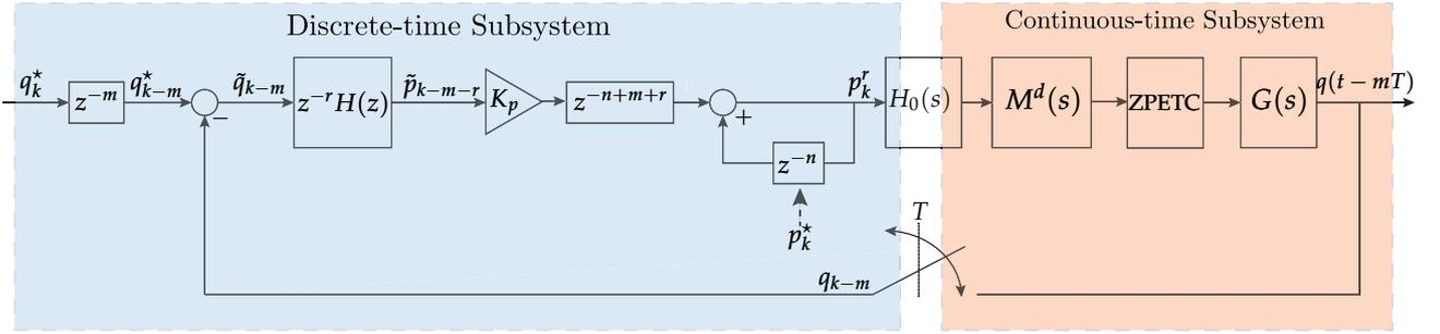
FIGURE 4.5: Discrete-time repetitive control scheme based on dynamic B-spline filter.
