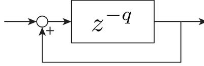
FIGURE 3.3: Discrete-time representation of the controller (3.3) for  $\mathcal{I} = \mathcal{H} = \mathcal{K} = I$ . It coincides with the digital version of the repetitive compensator present in RC schemes. Here  $z^{-1}$  represents the one-step delay operator.
