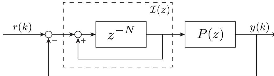
FIGURE 1.7: Discrete-time RC scheme.
