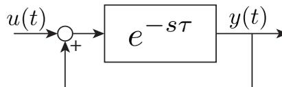
FIGURE 2.2: The repetitive compensator with I/O signals.
