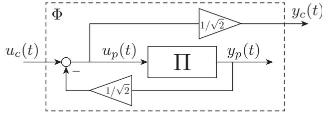
FIGURE 2.11: System (2.86) with the input / output Cayley transformation
