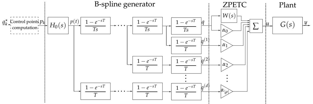
FIGURE 4.2: Block-scheme representation of feedforward control based on B-spline trajectory and CZPETC ( $d = |\rho|$ ) for the plant  $G(s)$ .
