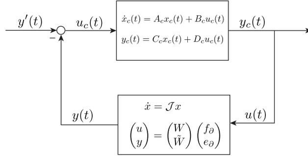
FIGURE 2.1: Standard feedback interconnection (2.10) of a finite dimensional controller (2.9) and a BCS defined in Theorem 2.1.1.
