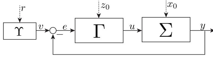
FIGURE 3.1: A graphical representation of the autonomous closed-loop system.
