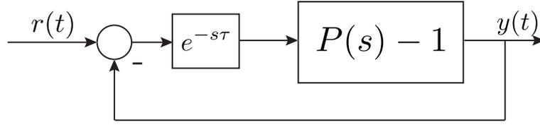
FIGURE 1.3: Equivalent scheme of RC for stability analysis.
