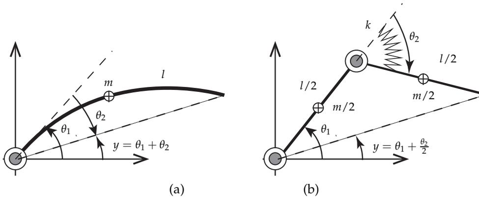
FIGURE 4.8: One-link flexible arm (a) and equivalent model with the deformation concentrated in an elastic hinge (b).
