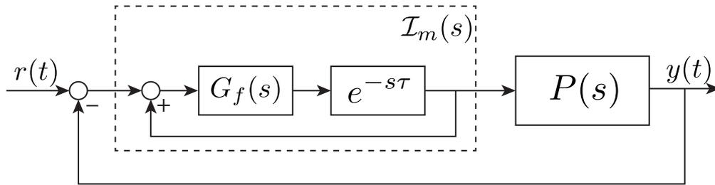
FIGURE 1.5: Continuous-time modified RC scheme.
