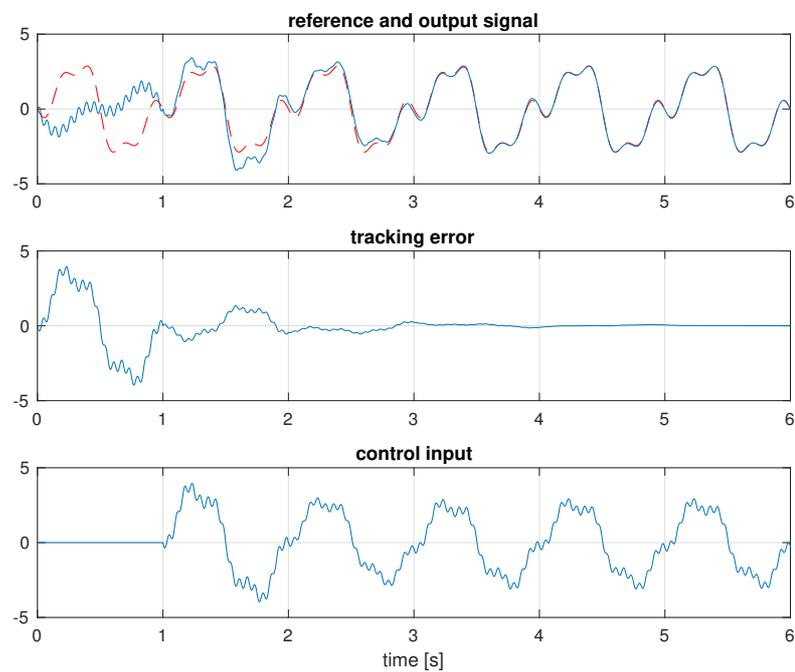
FIGURE 2.12: Asymptotic tracking and disturbance rejection of the RC system in which  $\Phi$  is the plant depicted in Fig. 2.11. In (2.86), we have selected  $S = 1.5$  and  $d(v_2) = 5v_2^3$ : with these choices the transformed system  $\Phi$  fits in (2.80).
