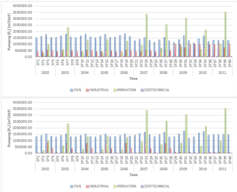
Figure 4.8: Total pumping ( $m^3/day$ ) insisting on the phreatic ( $P_1$ ) and confined ( $P_2$ ) aquifer for different uses for each stress period ( $SP$ ).
