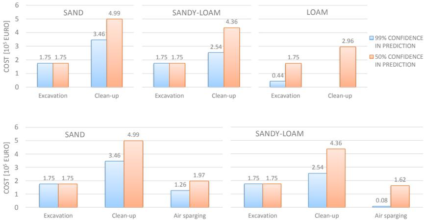
Figure 3.4: The 50% and 99% probability estimates of the overall costs of subsurface remediation in Scenarios 1 (top) and 2 (bottom).
