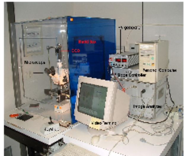
Figure 3.8: Left: Hardware configuration of the SAMAICA system. Right: Set up of the measuring system at the laboratory of the INFN Bologna.
