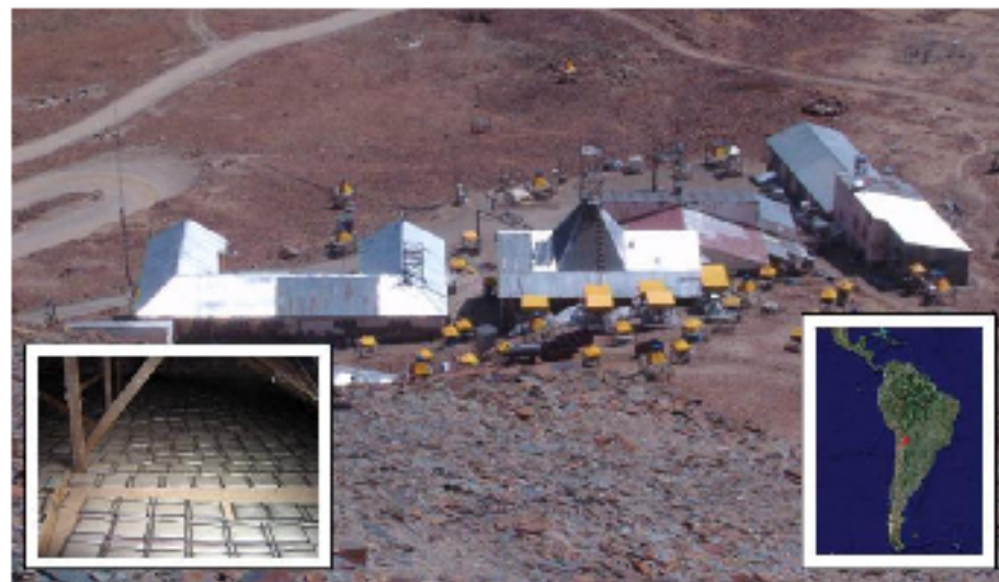
Figure 4.1: The Chacaltaya high altitude laboratory. The NTDs were placed on the roof of the buildings (at \sim 4 m from the ground level), as shown in the photograph on the left corner of the composition. The geographical position of the lab. is 16^{\circ}\text{S } 68^{\circ}\text{W} , and is indicated on the right corner.
