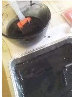
Figure 6.4: graphene based compound before the casting and curing
