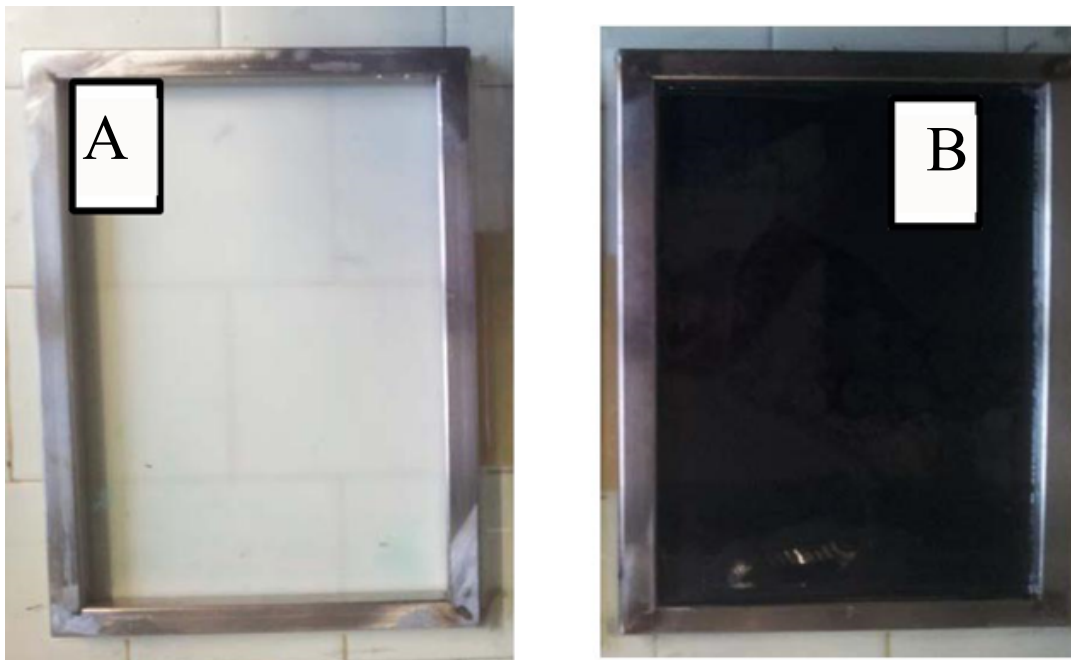
Figure 6.6: Picture of (A) metallic frame (200 x 270 mm) and (B) GNP-resin composite cast in the metallic frame
