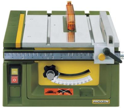
Figure 7.21: Proxxon FET used to create the V-notch in fracture toughness sample
