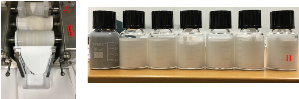
Figure 6.16: A) BN-PDMS compound milled with three roll milling; (B) different bottle of not cured PDMS with different concentration of boron nitride and graphene nano-platelets
