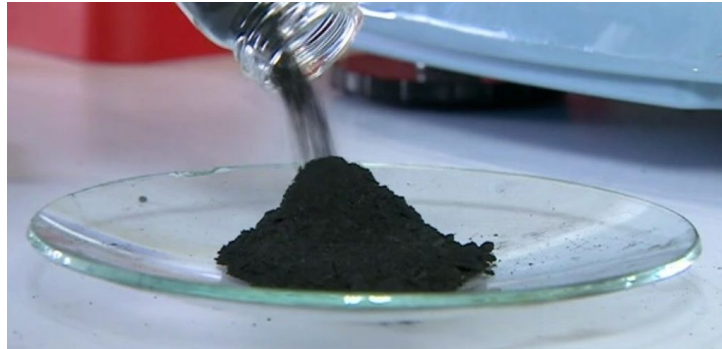
Figure 6.2: graphene related material, black volatile powder
