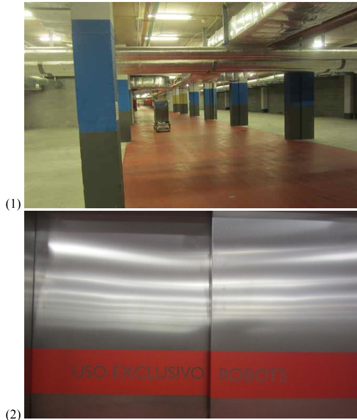
Figure 23 Exclusive Robot Corridor (1) and Robot Elevator (2) where you can read in Spanish “Robots exclusive use”. Own photography.
