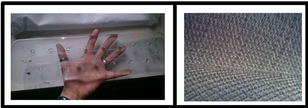
Figure 3.15: Milling machining tests. 1 of 2 layers treated: on the left the assembled 2 layer channel, on the right the picture under microscope of the treated layer.
