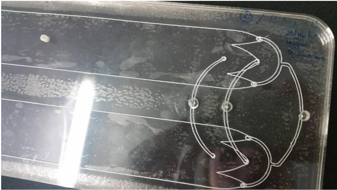
Figure 3.17: Sedimentation of salts on the edges of biadhesive layers
