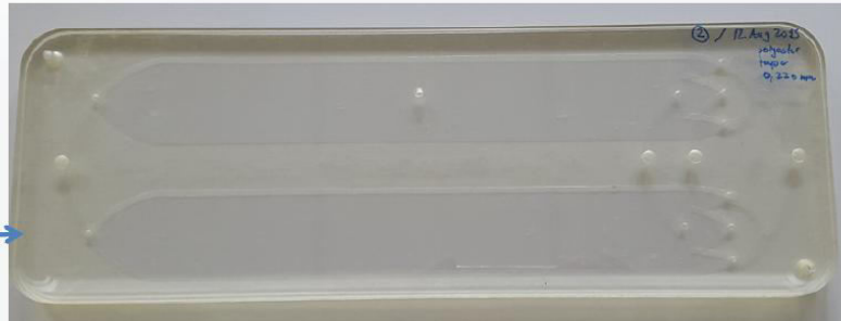
Figure 3.16: Prototypes of self-sustained channel. The thin PMMA layers are replaced by (1) Acrylic foam and (2) polyester biadhesive tape layers of the same thickness respect to PMMA layers.
