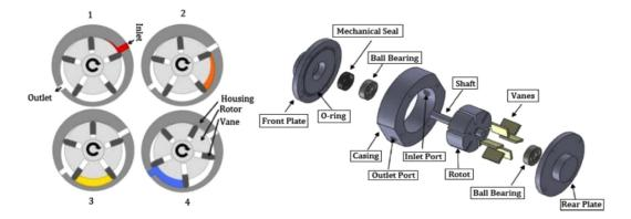
Fig. 7.7: Working principle and components of vane expander [93].
