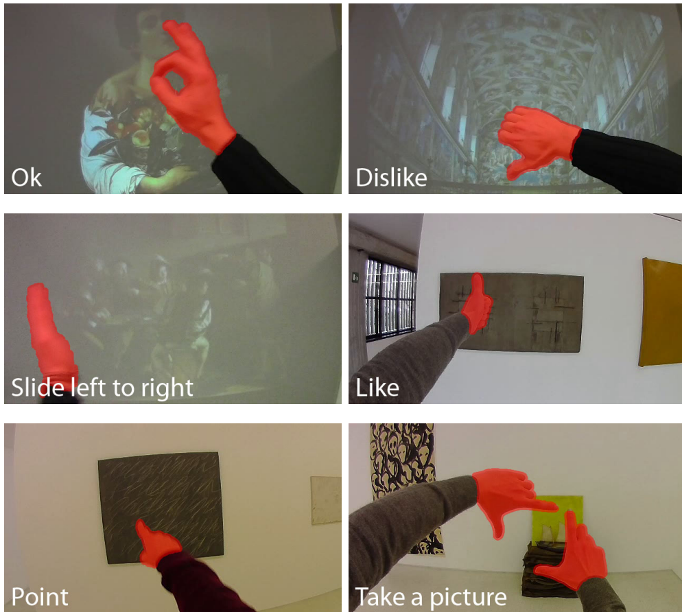
Figure 3.1: Natural interaction with artworks: visitors can get specific content or share information about the observed artwork through simple gestures. Hand segmentation results are highlighted in red and detected gestures are reported in the bottom part of each frame.
