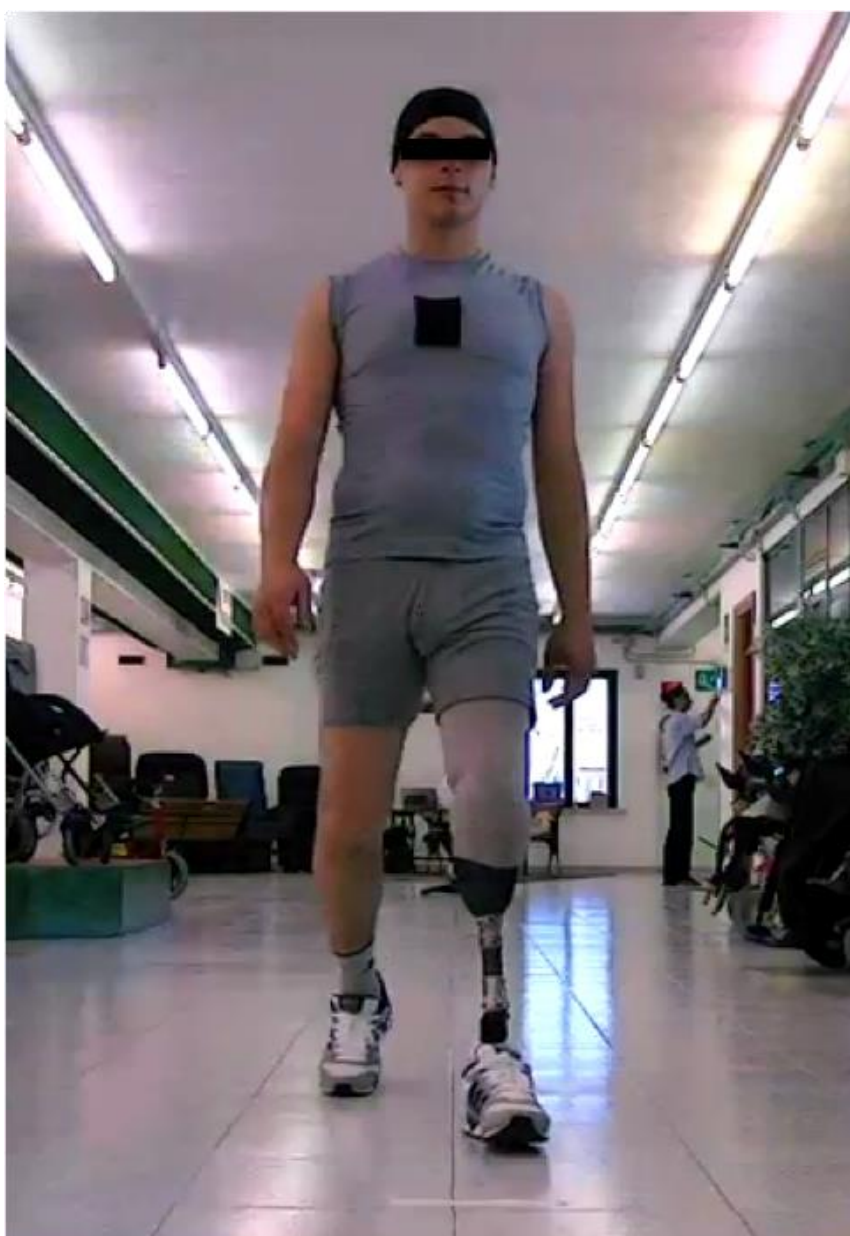
Figure 5.2 – Execution of the walking test. Note the pocket on the stretch top for housing the measurement unit on the sternum.
