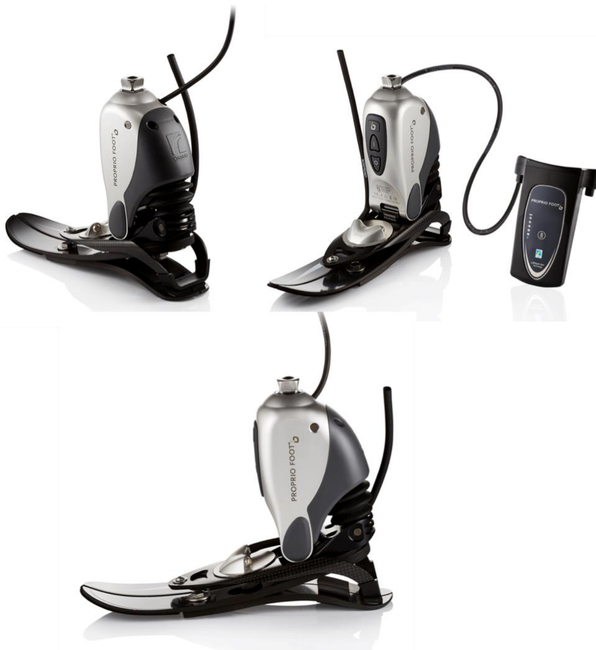
Figure 7.1 - The electronic ankle Proprio Foot microcontrolling based (Össur, Reykjavik). It is an adaptive prosthetic device for low to moderately active below-knee amputees that mimics natural foot motion. It has a rechargeable lithium-ion battery (1800 mAh) with output voltage = 14.8 V.
