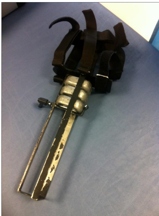
Figure 8.2 - The system specifically designed and developed for the study. It allows the modular application of loads distally, minimizing measurement errors due to the knee flexion. Each weight is 1 kg ( \approx 1\text{N} ), with a mobile guide at the bottom.
