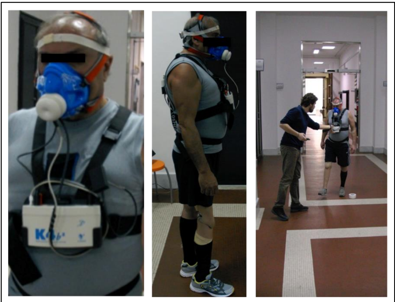
Figure 9.10 - The Six-Minute Walking Test instrumented with a gas analyzer, an heart rate monitor and three MIMU.
