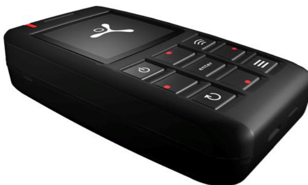
Figure 4.1 – The FreeSense (Sensorize) inertial system. This unit contains a 3-axial accelerometer ( \pm 6g ), a 3-axial gyroscope ( \pm 500 deg/s), and a GPS module along with a wireless transmission module for sending data to a computer station and a memory card to store alternatively all data on board (sampling frequency = 100 Hz, weight = 93 g).
