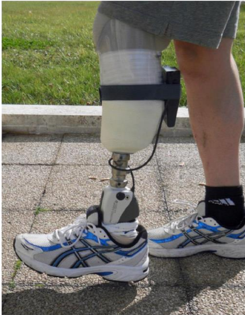
Figure 7.2 - The Proprio Foot during the swing phase automatically lifts the toe to reduce the risk of trips. Note the battery on the rear side of the socket and the Seal-In X5 liner under the test socket.
