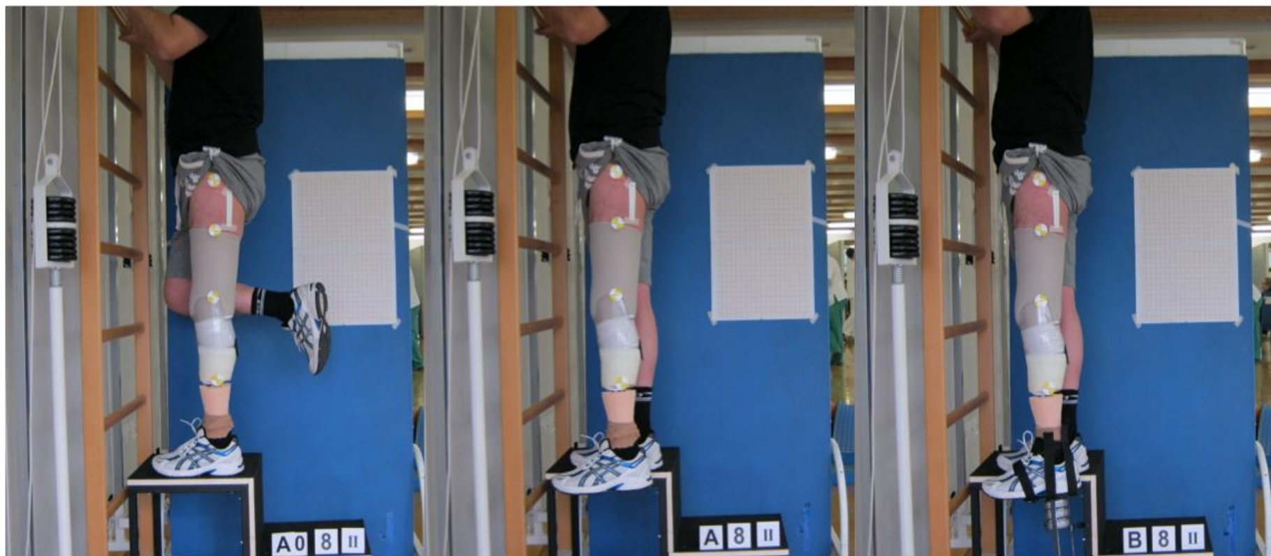
Figure 8.3 - The three conditions of the pistoning test on the hypobaric Icross Seal-In X5. The baseline evaluation is on the left, 0 N applied to the prosthesis is in the middle, and 30 N applied is on the right. Note the markers on the thigh and on the socket.
