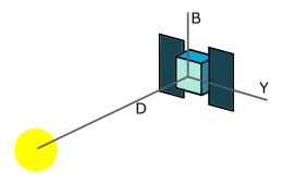
Figure 2.3 – Scheme of the satellite-Sun oriented frame: the D-axis is the satellite-Sun direction (i.e. it is normal to the plane in which the solar panels lie), the Y-axis is the rotation axis of the solar panels and the B-axis completes the right-handed triad.
