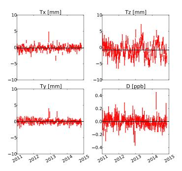
Figure 3.6 – Translation and scale offsets estimated between the frames realized, on a weekly basis, by a LAGEOS-only solution and by the SLR subnetwork of the fully combined adjustment -  $CASE\ A$ .
