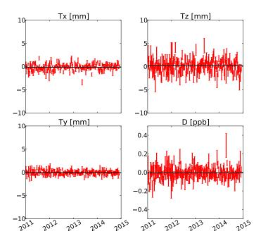
Figure 3.7 – Translation and scale offsets estimated between the frames realized, on a weekly basis, by a LAGEOS-only solution and by the SLR subnetwork of the fully combined adjustment -  $CASE\ B$ .
