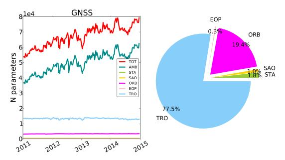
Figure A.3 – Panlel a): number of parameters estimated in GNSS analysis; panel b): pie chart displaying the relative abundance of set-up parameters excluding initial-phase ambiguities.
