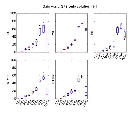
Figure B.2 – Relative improvement in the formal errors of empirical orbit parameters with respect to a GPS-only solution. The characteristics of displayed cases are detailed in Tab. 3.7.
