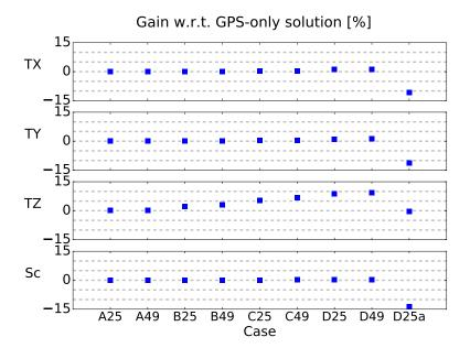
Figure 3.10 – Relative improvement in the formal errors of reference frame parameters with respect to a GPS-only solution, see Tab. 3.9, first column. The characteristics of displayed cases are detailed in Tab. 3.7.
