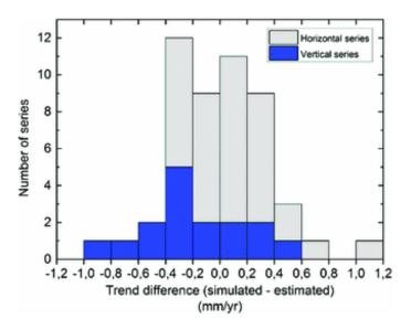
Figure C.4 – Comparison between the originally simulated trends and the velocities of the corrected time series. Vertical-like time series are shown in blue, while horizontal-like data sets are shown in gray
