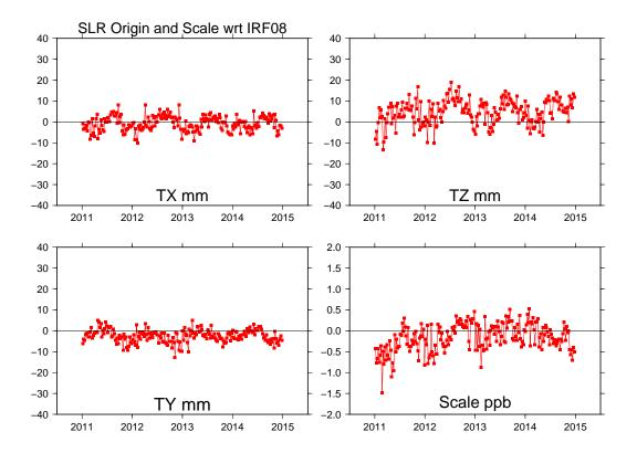
Figure 2.16 – Translation and scale offsets computed during the long term stacking of SLRtoLAGEOS weekly solutions. MC have been imposed with reference to ITRF2008.
