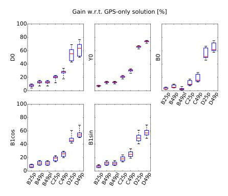
Figure B.6 – Relative improvement in the formal errors of empirical orbit parameters with respect to a GPS-only solution encompassing the estimation of zPCOs. The characteristics of displayed cases are detailed in Tab. 3.7.
