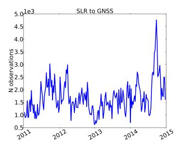
Figure 2.17 – Number of SLR observations to GNSS satellites for each 9-day solution. A clear acquisition increment is observed starting from August 2014 coinciding with the beginning of the first LARGE experiment.
