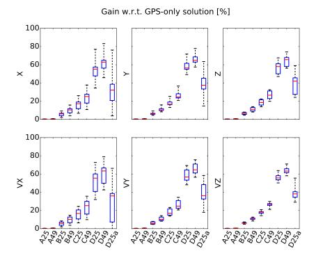
Figure B.1 – Relative improvement in the formal errors of orbital parameters (initial state vector) with respect to a GPS-only solution. The characteristics of displayed cases are detailed in Tab. 3.7.
