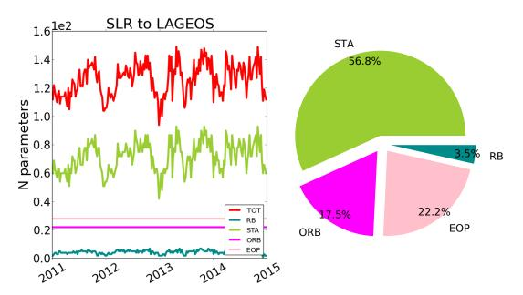
Figure A.4 – Panlel a): number of parameters estimated in the SLR analysis of LAGEOS observations; panel b): pie chart displaying the relative abundance of set-up parameters.
