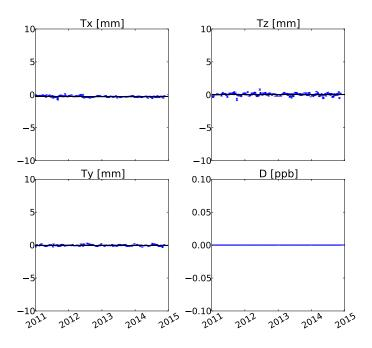
Figure 3.4 – Translation and scale offsets estimated between the frames realized, on a weekly basis, by a GNSS-only solution and by the GNSS subnetwork of the fully combined adjustment.
