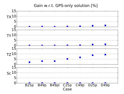
Figure 3.12 – Relative improvement in the formal errors of reference frame parameters with respect to a GPS-only solution encompassing the estimation of zPCOs, see Tab. 3.9, third column. The characteristics of displayed cases are detailed in Tab. 3.7.
