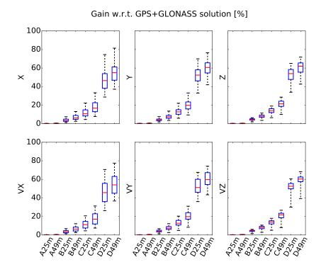
Figure B.3 – Relative improvement in the formal errors of orbital parameters (initial state vector) with respect to a GPS+GLONASS solution. The characteristics of displayed cases are detailed in Tab. 3.7.
