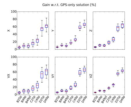
Figure B.5 – Relative improvement in the formal errors of orbital parameters (initial state vector) with respect to a GPS-only solution. The characteristics of displayed cases are detailed in Tab. 3.7.
