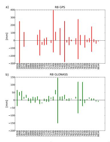
Figure 3.9 – Range biases estimated from the long term stacking of fully combined weekly frames derived from *CASE B* solutions, see Sec. 3.3. RBs are estimated per station and group of satellites, results concerning the two GPS spacecrafts equipped with retro-reflector arrays are presented in panel a, while the analogous results for all GLONASS vehicles are shown in panel b. Error bars are consistently estimated during the stacking.
