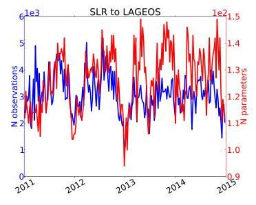
Figure 2.12 – Number of observations (blue line - left axis) and of estimated parameters (red line - right axis) for each weekly SLRtoLAGEOS solution.
