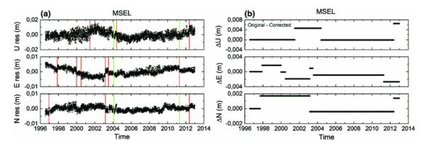
Figure C.9 – MSEL station: a Up, East and North residuals of the original GPS coordinate time series. Red lines indicate the detected discontinuities; green lines indicate the firmware upgrade and the change of the reference system. b Difference between the original and the corrected Up, East and North coordinate time series; the scales are different from those of panel a to clearly distinguish the magnitude of the discontinuities
