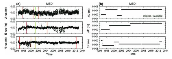
Figure C.10 – MEDI station: a Up, East and North residuals of the original GPS coordinate time series. Red lines indicate the detected discontinuities; the green line indicates the antenna and receiver change. b Difference between the original and the corrected Up, East and North coordinate time series; the scales are different from those of panel a to clearly distinguish the magnitude of the discontinuities
