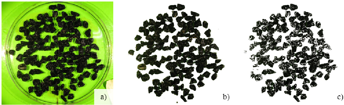
Figure 7.2: Image filtering process. a) original image; b) non-classified image; c) classified image
