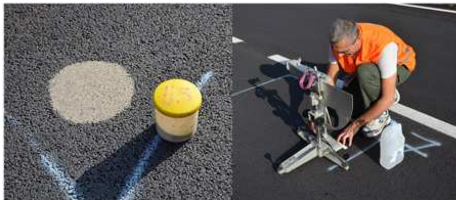
Figure 5.12: BPN measured at different locations during the surveys for SMA 0
