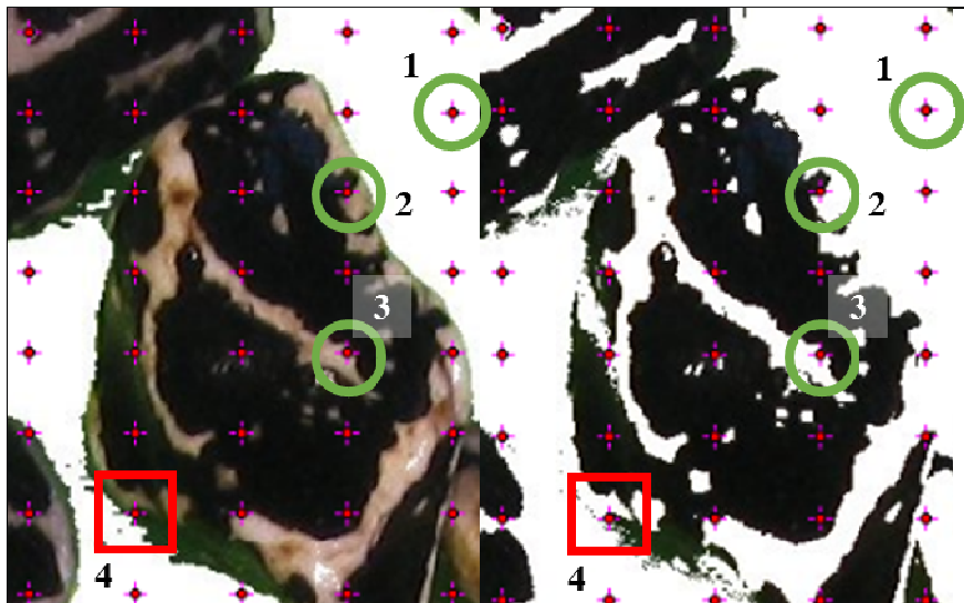
Figure 7.4: Detail of pixels' colour inspection: correct and incorrect classifications
