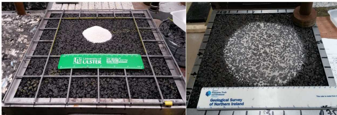
Figure 6.4: Sand placed onto the surface (left) and evenly spread for measuring MTD
