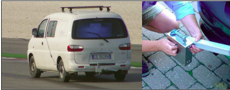
Figure 5.29: Laseprof equipment for MPD survey
