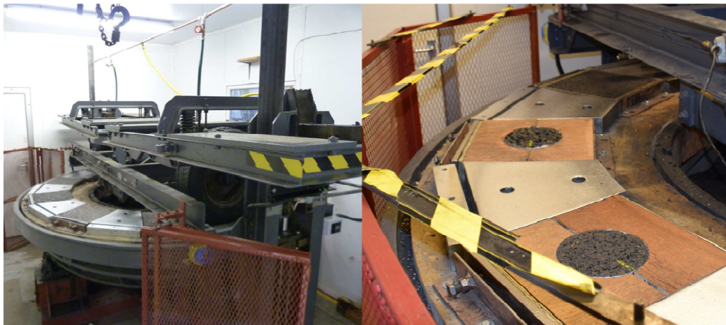
Figure 6.1: Road Test Machine
