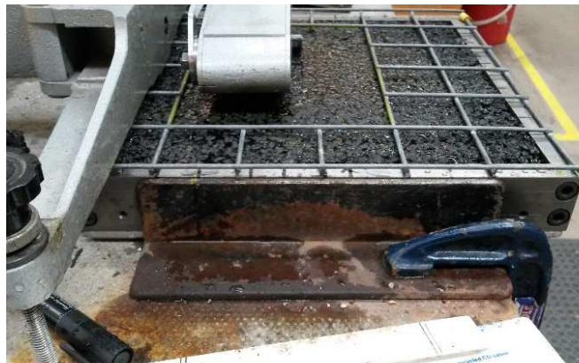
Figure 6.7: Steel frame for detecting the area of testing
