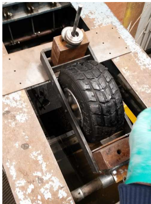
Figure 6.3: Treaded tyre used for the Immersion Wheel Track
