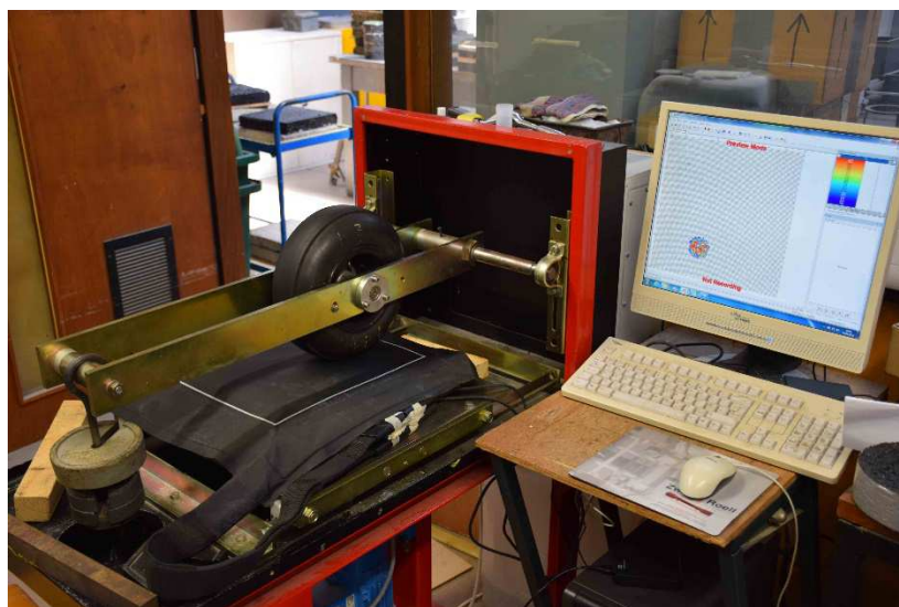
Figure 9.1: Equipment for the tyre/surface interaction analysis
