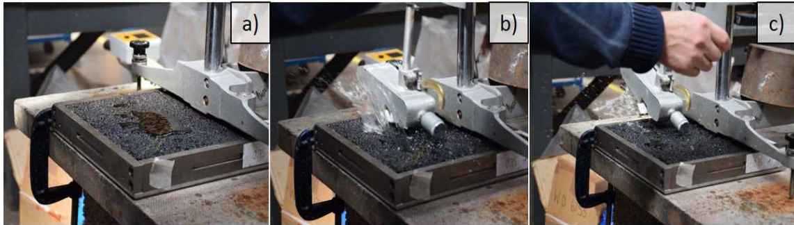
Figure 6.8: Pendulum test. a) the surface is free; b) the slider is in contact with the surface; c) the arm is hold before it swings back to the surface
