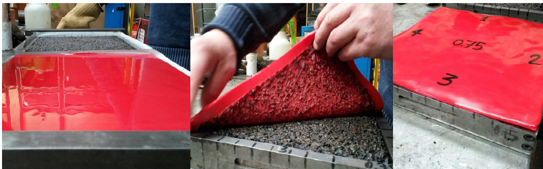
Figure 8.70: Peeling off the hot vinamold from the slab surface
