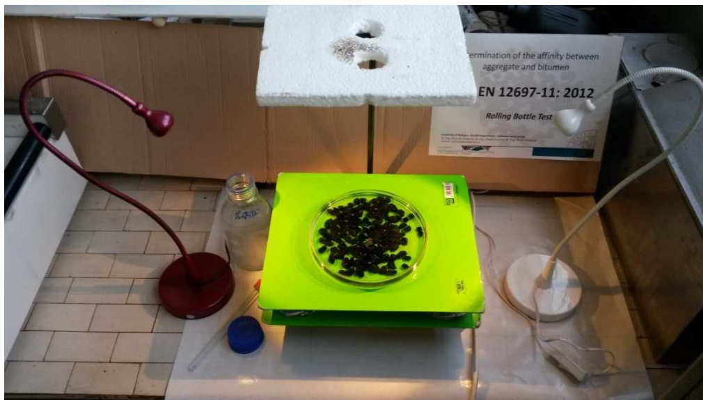
Figure 7.1: Set for digital picturing of tested samples
