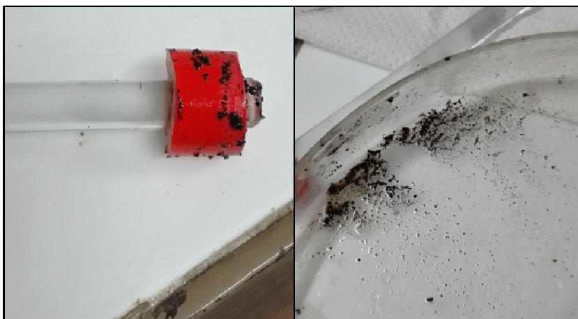
Figure 7.7: Loss of rubber during the Rolling Bottle test
