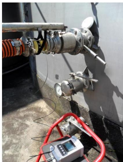
**Figure 3.6.** PSt3 sensor in specula used to monitor the DO during wine transport.
