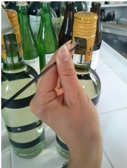
**Figure 2.13.** The measurement of head space oxygen with the colorimetric after Nomacorc.
