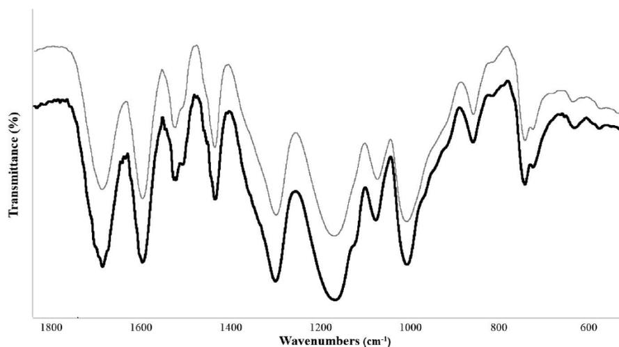
FIG. 6. Comparison between gallnut extract (gray line) and sample HY-GEN2, a hydrolyzable tannin (black line).
