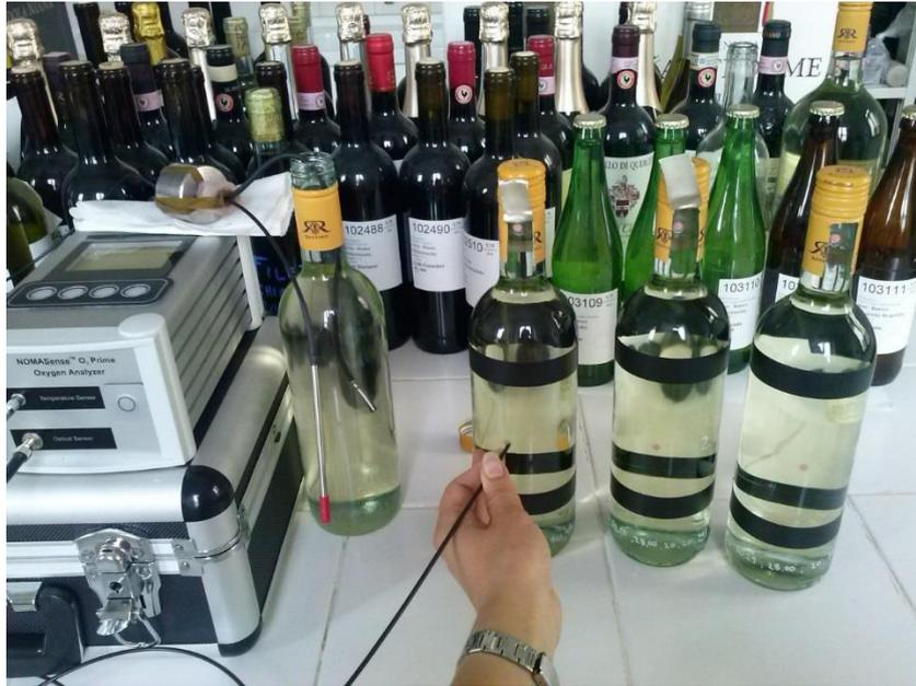
**Figure 2.12.** The measurement of dissolved oxygen with the colorimetric method after Nomacorc (Limbourg-Dolhain, France).
