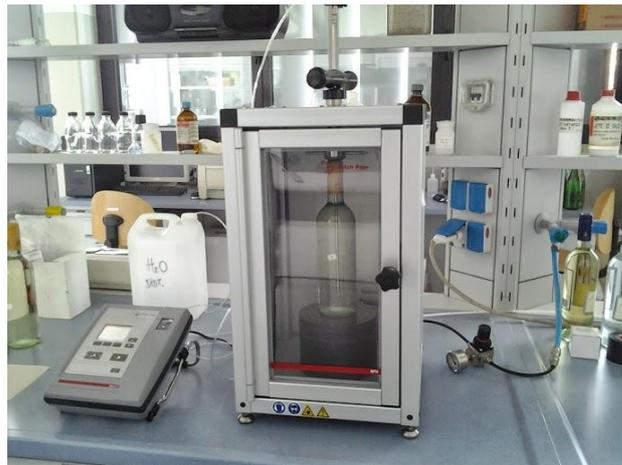
**Figure 2.14.** The sampling chamber to measure dissolved oxygen in bottled wines after AntonPaar (Graz, Austria).
