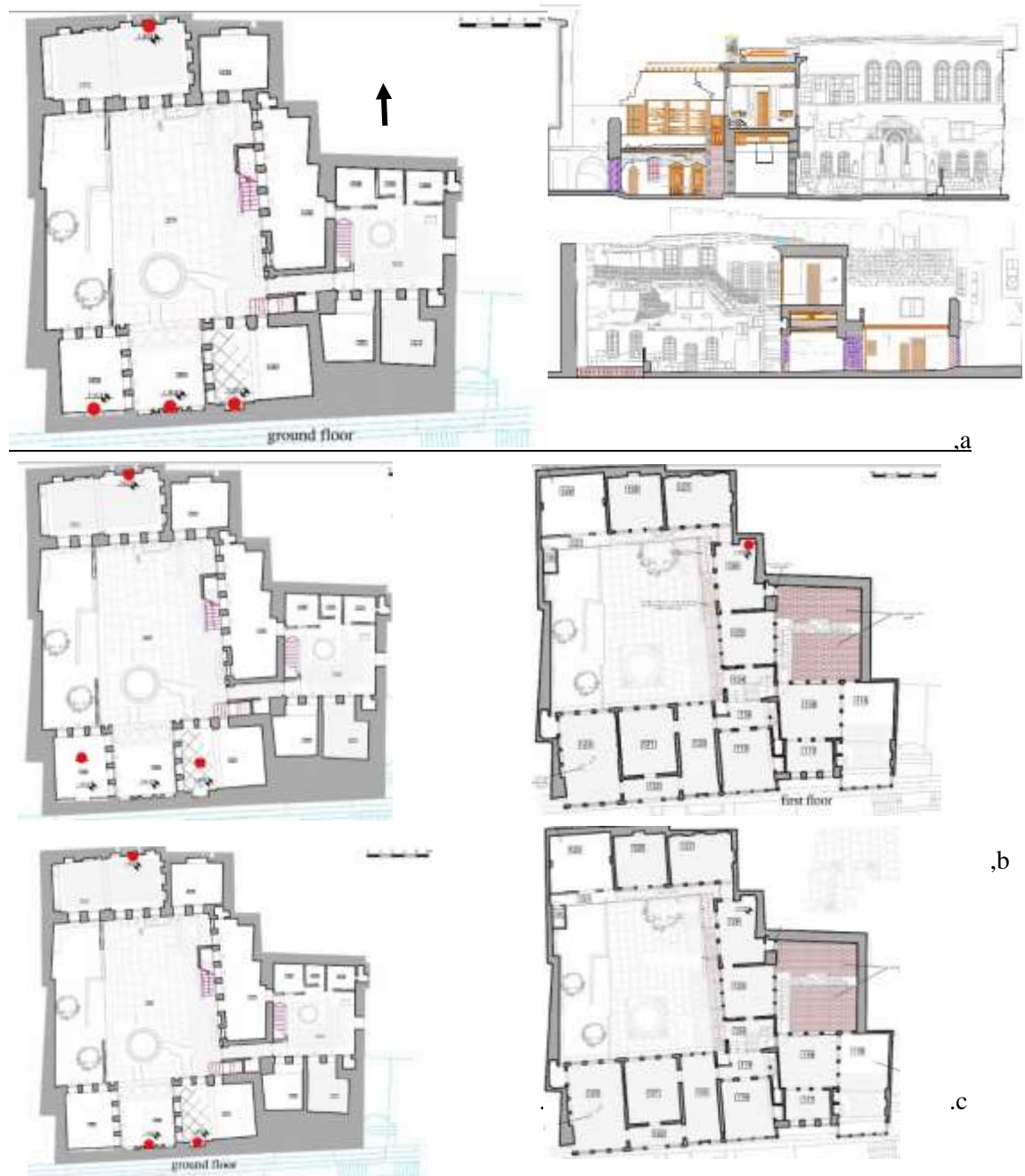
Figure C-10: Mouslli measurements stages instruments positions summer 2014 th , a .first stage, b .second stage .c. instruments position winter 2014 th /2015 th .
