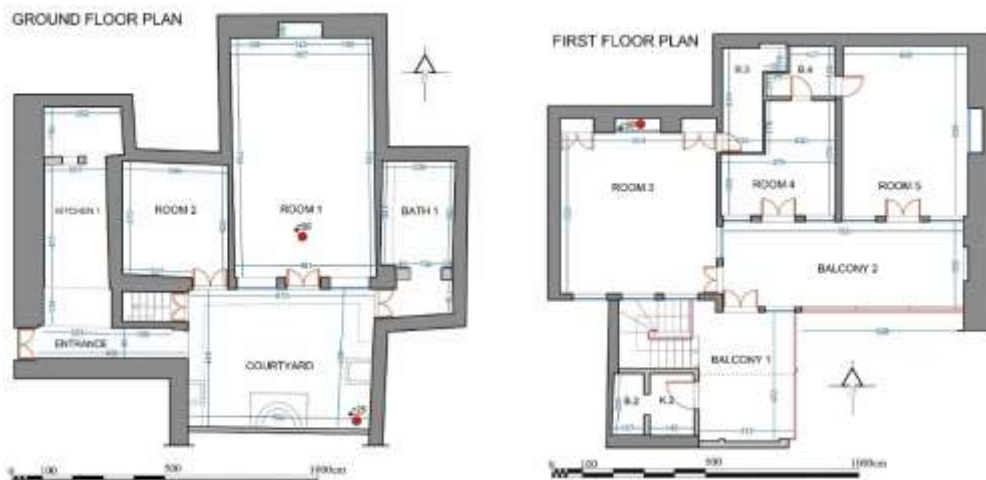
.a. BAB AL SALAM HOUSE plans and instruments positions .
