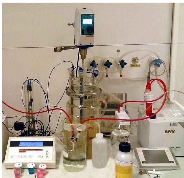
Fig. S4-1 Experimental setup of leaching procedure in a 2 litre glass reactor, equipped with titration system and benchtop meters for continuous monitor of pH, red-ox and temperature.
