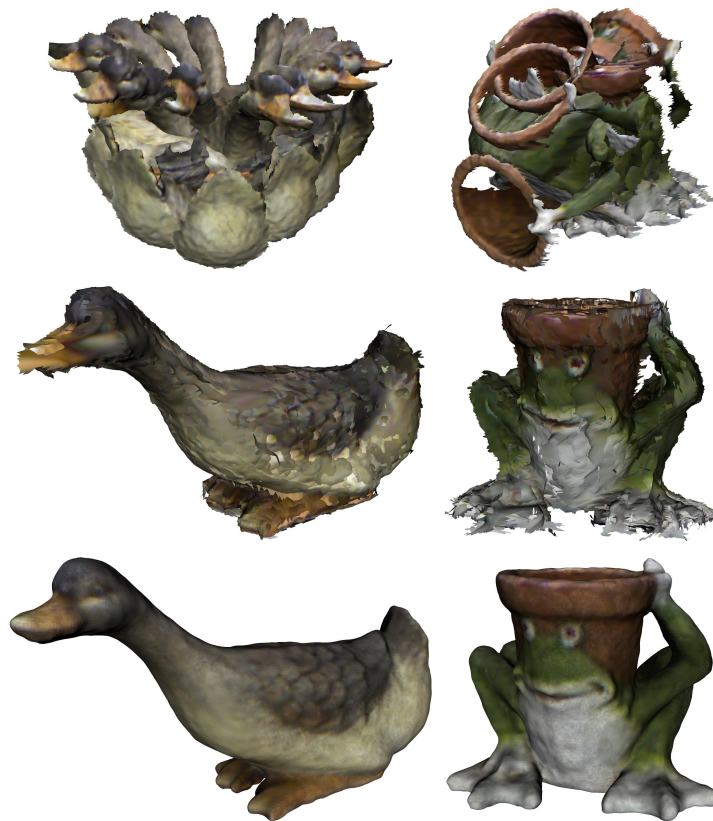
FIGURE 4.4: Reconstructions of DuckKinect and FrogKinect . Top: initial disarranged views. Center: coarse reconstructions provided by our pipeline. Bottom: final meshes attained by refining coarse reconstructions by Scanalyze and then running Poisson Reconstruction .
