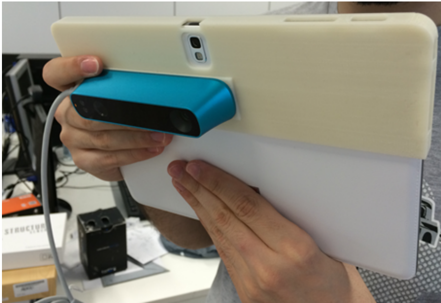
FIGURE 7.8: Structure Sensor clipped onto the Samsung tablet for the acquisition of the depth image.
