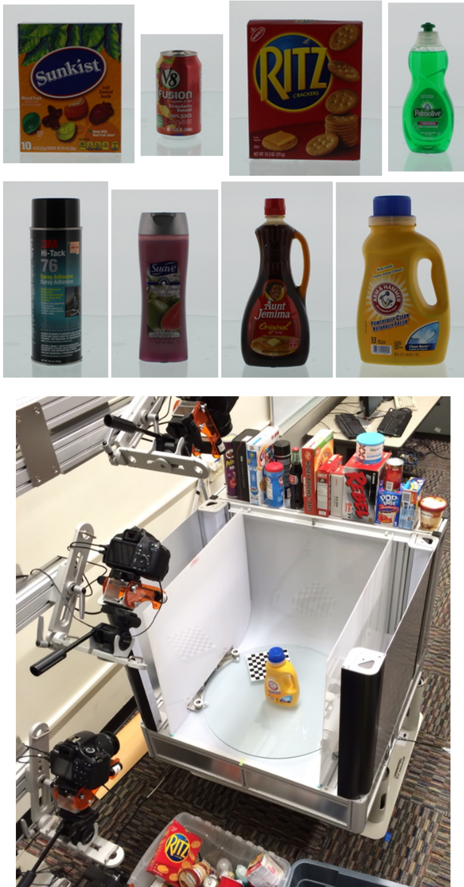
FIGURE 6.3: BigBIRD dataset. Top: examples of objects included in the dataset. Bottom: setup staged to acquire the dataset.
