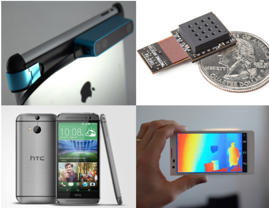
FIGURE 1.3: Examples of 3D sensing solutions for mobile devices. Top-left: the Structure sensor mounted on an iPad; top-right: the PiCam by Pelican Imaging ; bottom-left: the HTC One (M8) smartphone; bottom-right: a prototype Tango device by Google.
