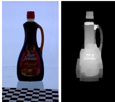
FIGURE 8.3: Example of saliency map. Brighter pixels represent more salient portions of the image.
