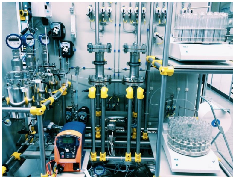
Figure 3.2 a). "Laboratory-Phenols-Adsorption-Reactor" of SIMA-tec GmbH (Schwalmtal, Germany), fot Ty and HTy adsorption (SIMA-tec).
