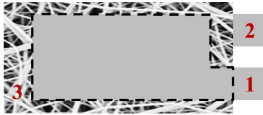
Figure 6.1 Example of tested sample: Electrodes (1, 2), electrospun piezoelectric sample (3); the dotted line surrounds the active area of the specimen.
