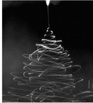
Figure 2.2 Taylor cone, linear path of polymeric jet and whipping instability during electrospinning [7].
