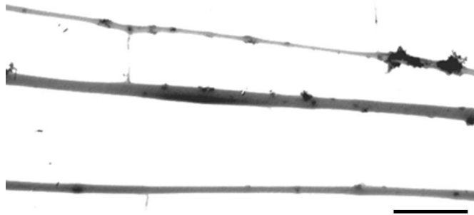
Figure 5.32 Fibers electrospun following protocol E: solution exposed to plasma (PRR = 1000 Hz, PV = 27 kV, treatment time = 3 minutes) after nanoparticle addition. Scale bar = 1 \mu m.
