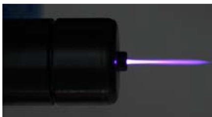
Figure 5.26 Picture of the plasma jet operated in Ar at flow rate 2 slpm, driven by the nanopulsed power generator, PRR 1000 Hz and PV 17 kV.
