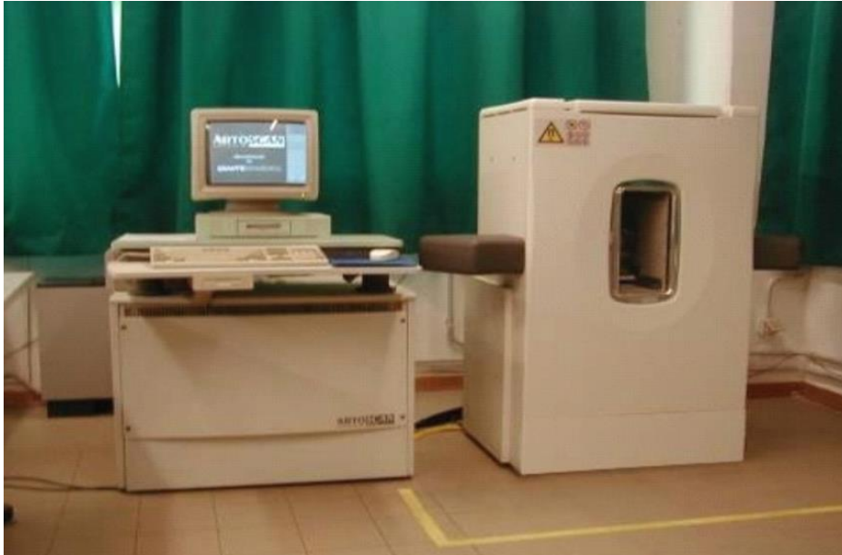
Figure 3.3: MRI apparatus based on the Artoscan Tomograph
