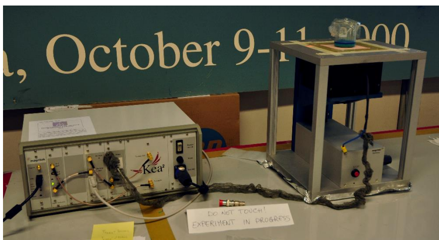
Figure 3.2: MOUSE PM10 mounted on a lift and KEA II spectrometer
