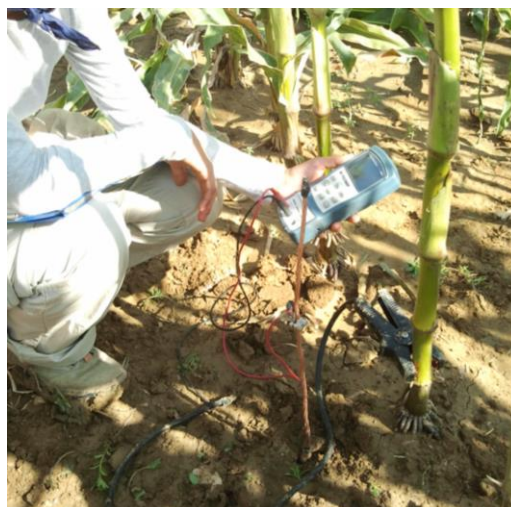
Figure 2. Root electrical capacitance measurement in the field using a portable capacitance meter (BK Precision 890C). The positive electrode is attached to a copper ground rod and the negative electrode is attached to the maize stem at 15cm above the ground.
