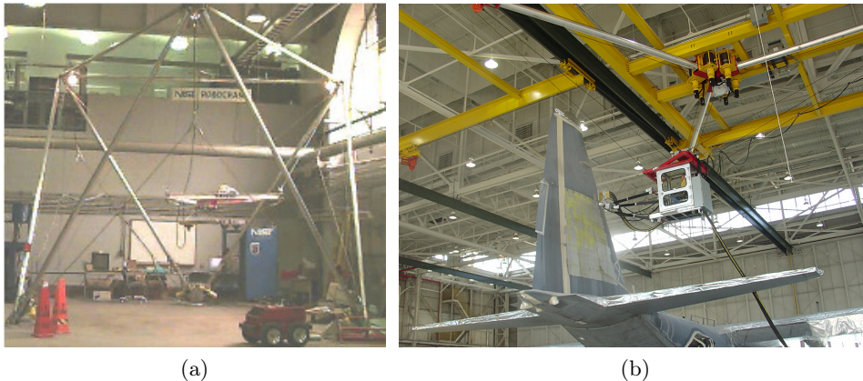
Figure 1.8 – On the left the first prototype of the NIST RoboCrane and on the right its version for aircraft painting and maintenance ([NIST 2006]).
