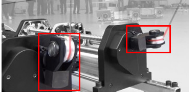
Figure 1.17 – A detail of the winches developed by the Fraunhofer Institute.
