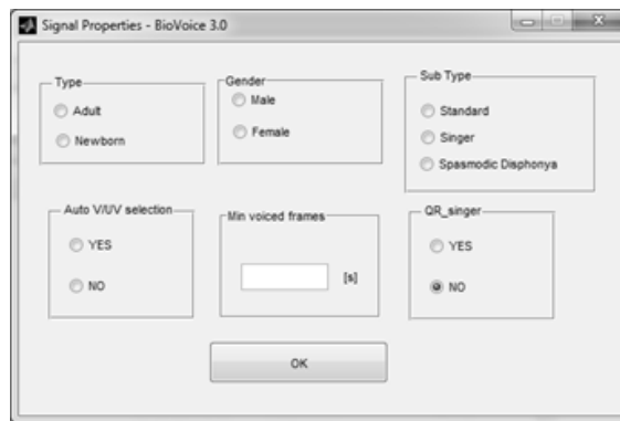
Figure 4.4 – BioVoice signal properties menu. The length of voiced frames can be selected by the user. For newborn cry the range is commonly set between 150 ms and 500 ms
