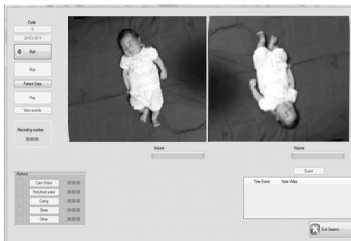
Figure 6.2. AVIM Recorder tool: acquisition window with a double view of the newborn. The user can select markers to point out the status of the patient (such as sleep, restlessness, etc.), ambient noise, interfering events and enter notes during the recording.
