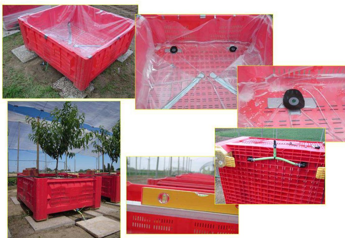
Picture 5.1. The lysimeters used in the experiment
