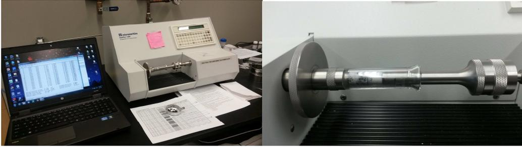
Picture 8.3. The Geopyc allowed the measurement of the particles envelope density. On the right, detail of the glass chamber where a sliding piston consolidated the pure DryFlo<sup>®</sup> around the biochar fragments
