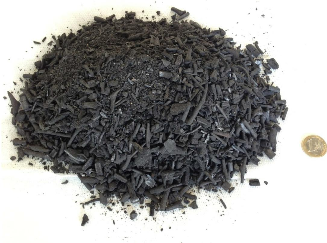
Figure 1.1. Biochar from hardwood pyrolyzed at 500 °C
