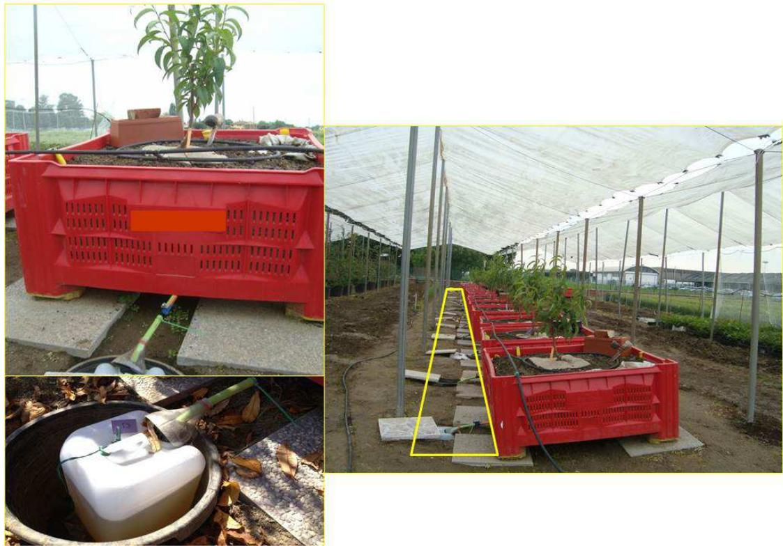
Picture 5.2. Leached soil solution was collected in tanks at the bottom of the lysimeters
