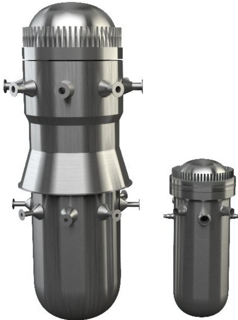
Figure 3-1: IRIS and AP1000 vessel comparison (Rhinceros 5)
