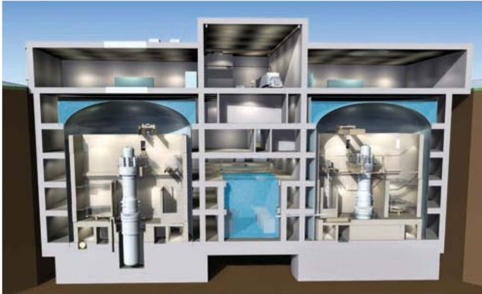
Figure 3-4: Two-Unit plant layout Figure and Containment building
