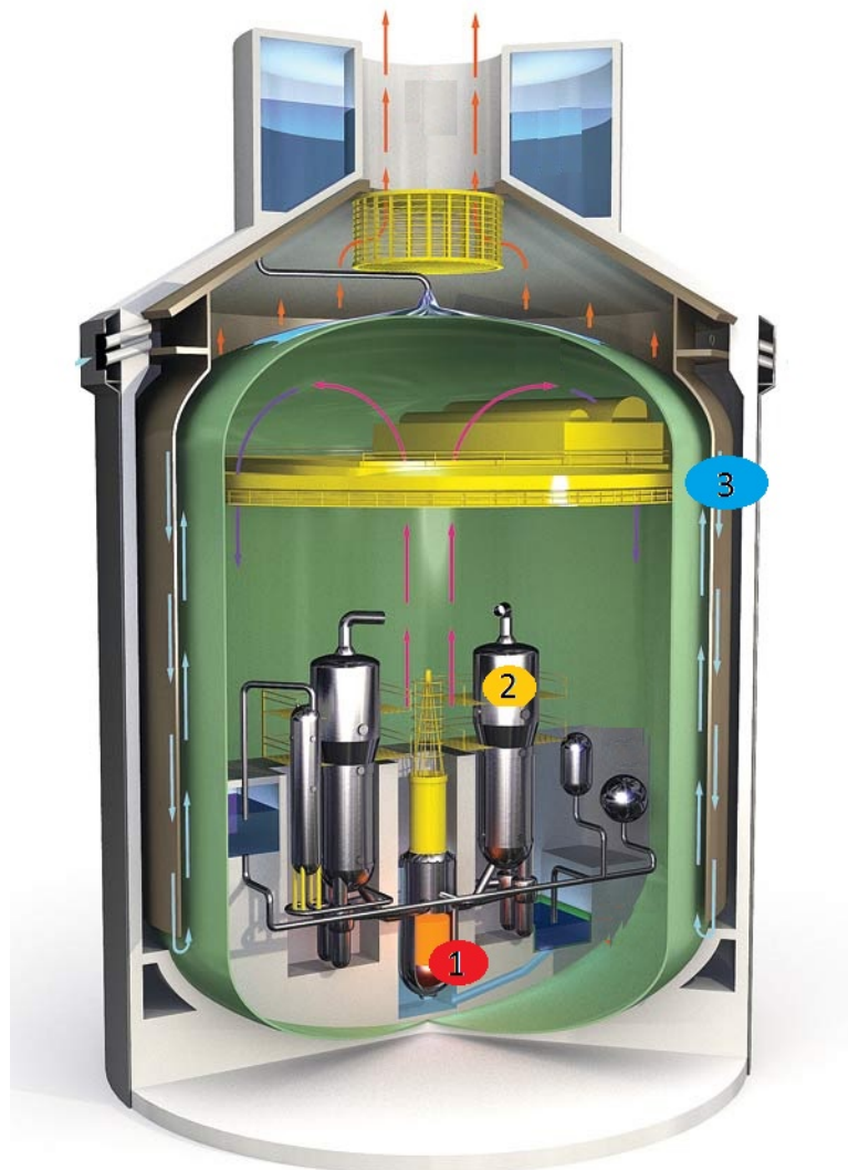
Figure 1-1: Physical Barriers for an AP1000 reactor
