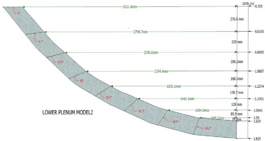
Figure 5-13: Lower head type 2 meshes
