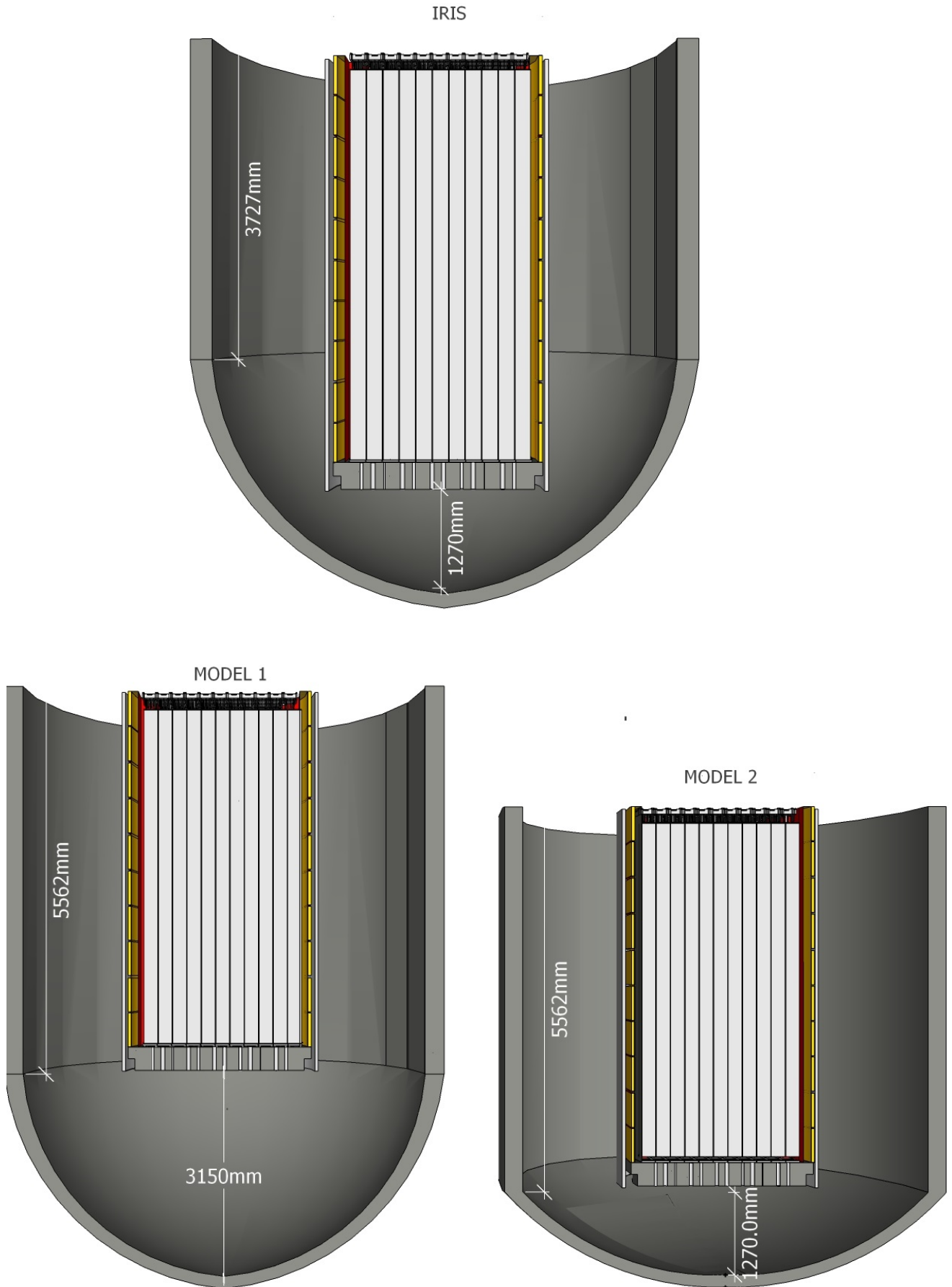
Figure A-1: IRIS lower head vessel and the two lower part vessel configuration
