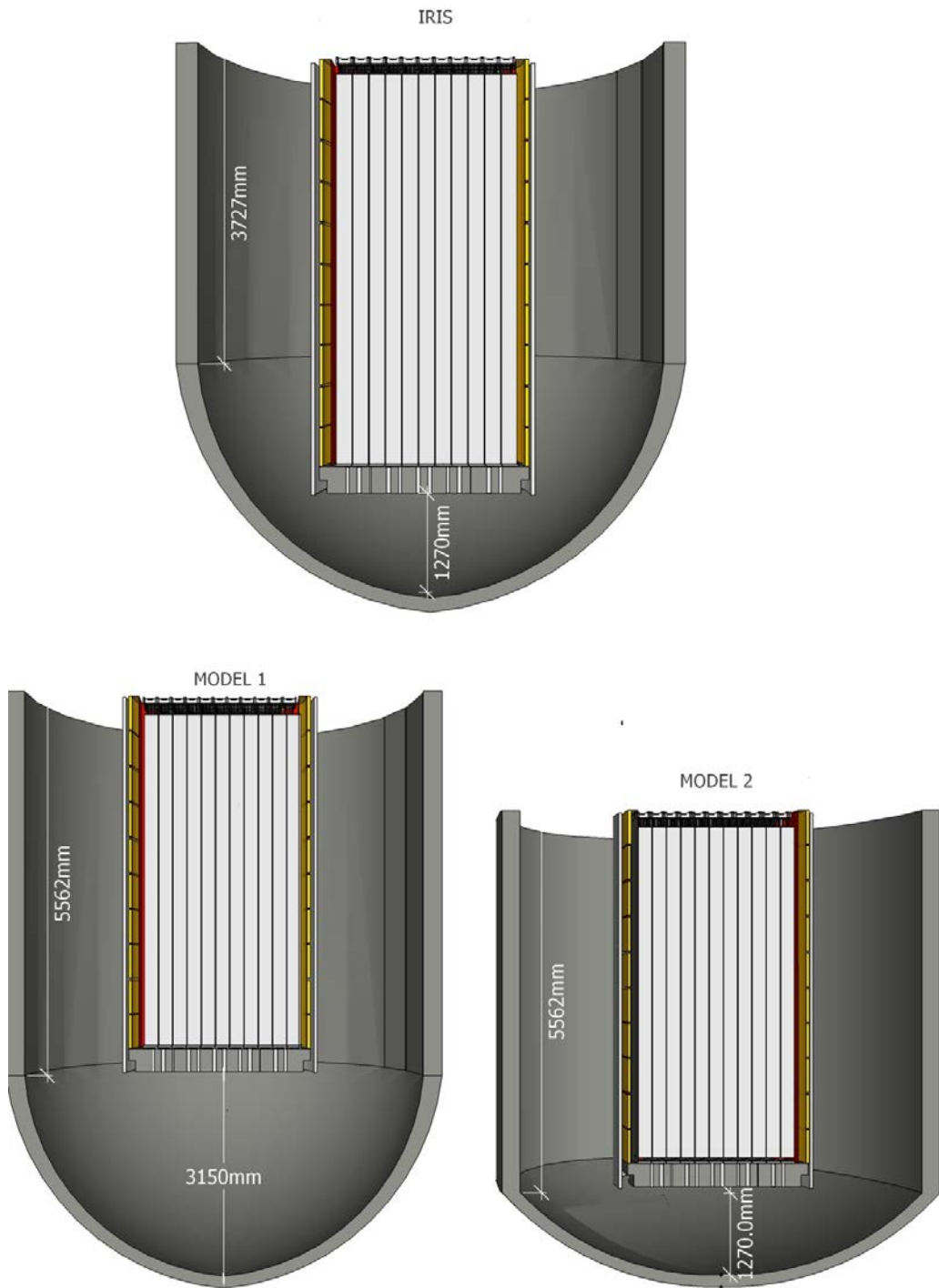
Figure 5-11: IRIS lower part vessel and the two lower part vessel models
