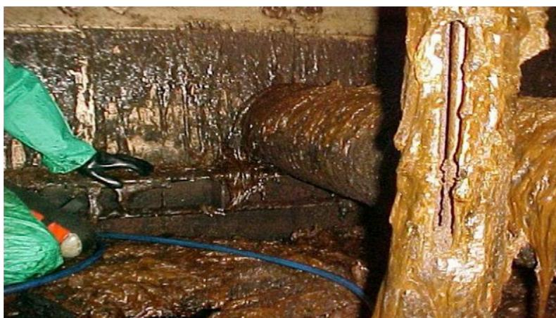
**Fig. 2.2.2 NA-mediated pipeline corrosion (Image courtesy of Oil Plus Ltd).**
