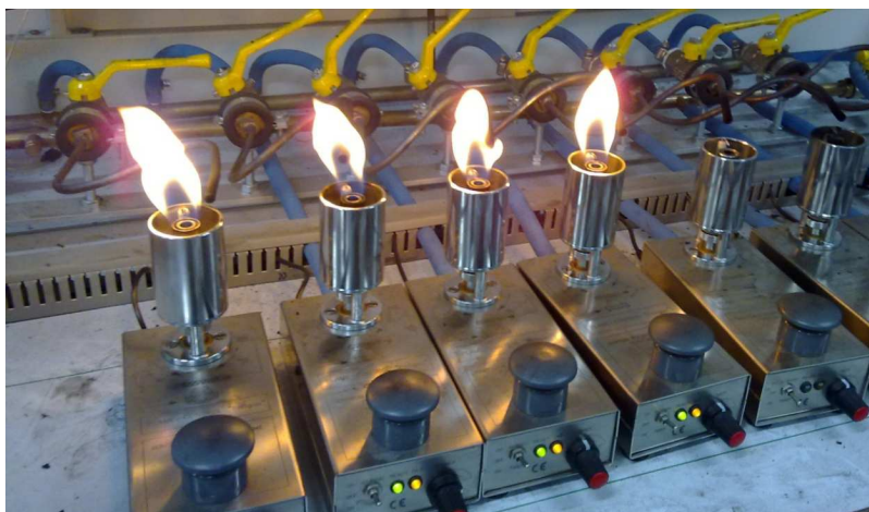
3.5 – An image of the first ignition of the syngas produced by pyrolysis of tires in the pilot plant.
