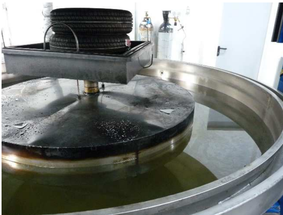
Figure 4.3 – Floating element inside the reactor.
