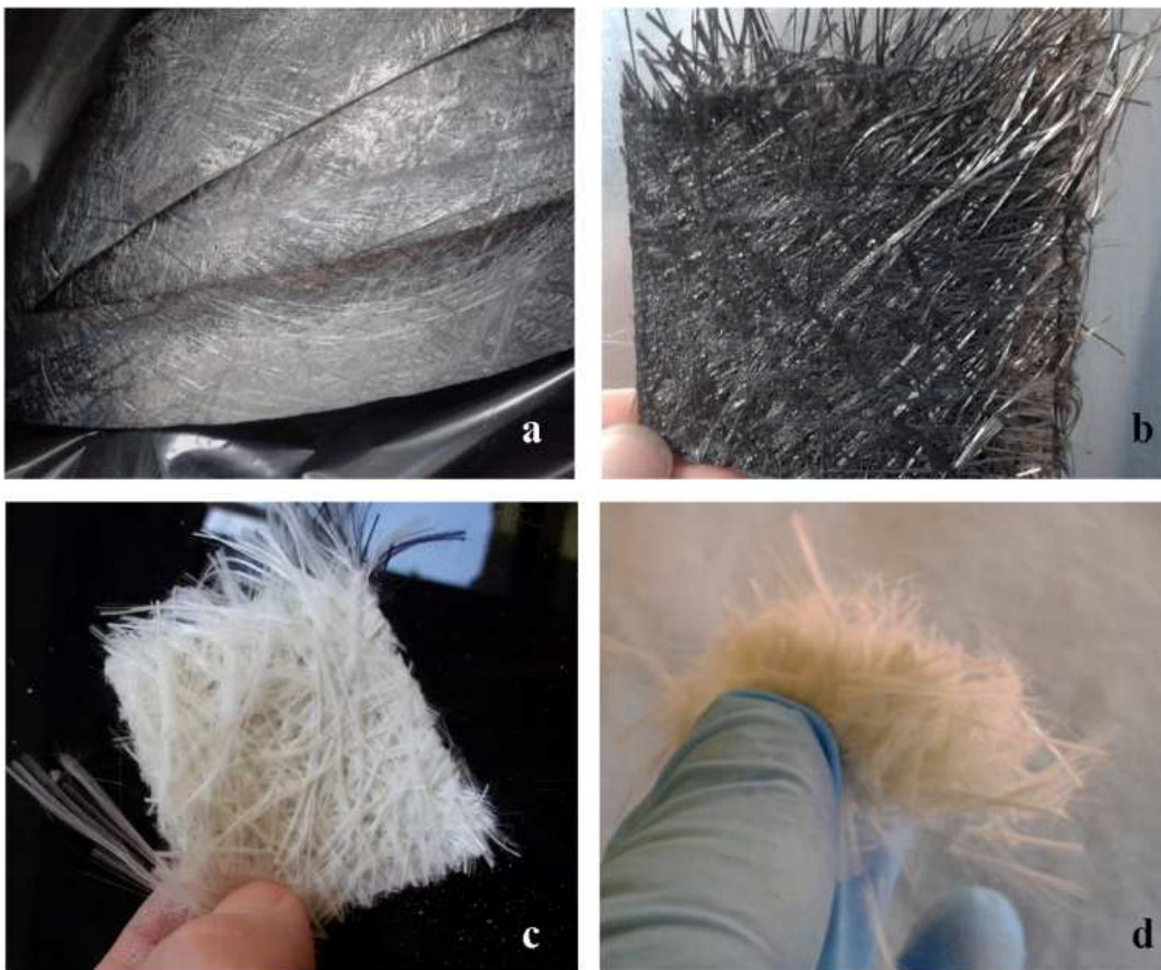
Figure 3.33 - Solid residue recovered from pyrolysis batches (a, b) and clean recovered glass fibers after oxidation to remove the carbonaceous layer (c, d).
