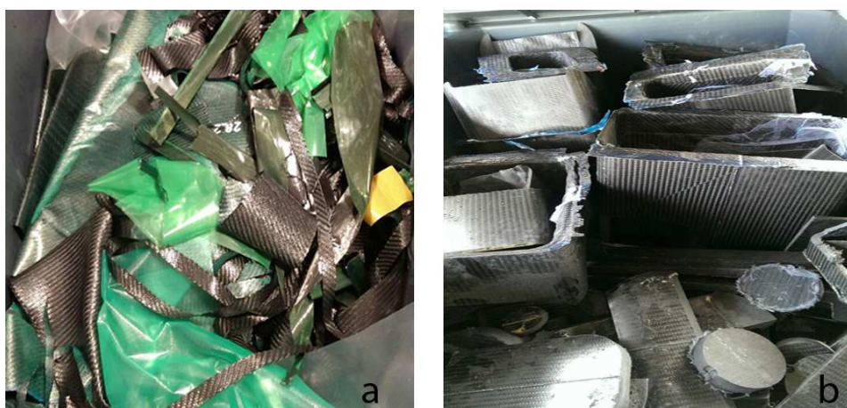
Figure 3.17 - Typical prepregs with LDPE protective film (a) and typical cured scraps of thick carbon fiber composites (b) [66]. Reproduced by permission of Wiley.
