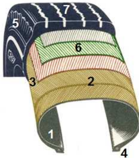
Figure 1.3 - Radial structure of a tire.
