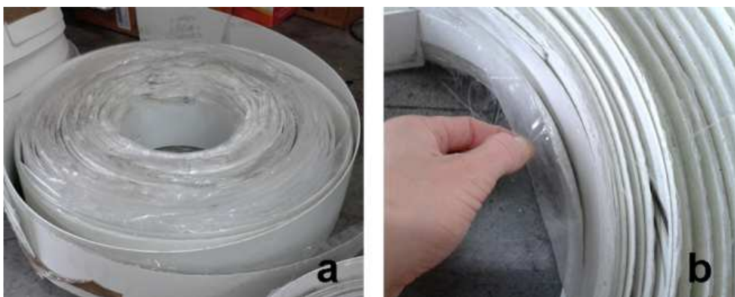
Figure 3.29 - Typical glass fibers reinforced polyester resin laminate scraps (a) and a focus on LDPE protective film (b).
