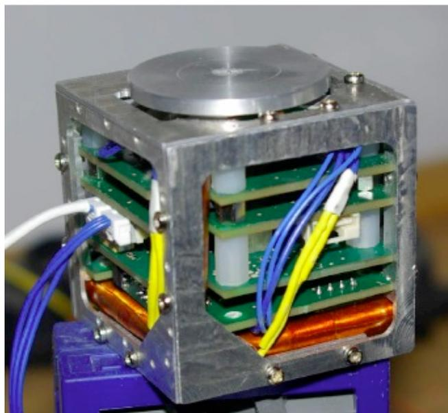
Figure III.2-2: Attitude determination and control system for Cubesat ([24])
