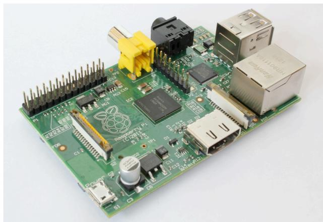
Figure V.2-1: Raspberry Pi (Copyright Raspberry Pi Foundation)
