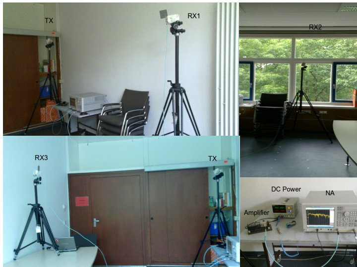
(b) The measurement room photo.
