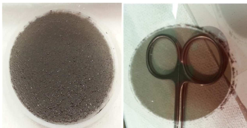
Fig. 4: HiPCO-SWCNT film (left) during dissolution of the alumina membrane and (right) after deposition in PS and dried in the oven overnight.
