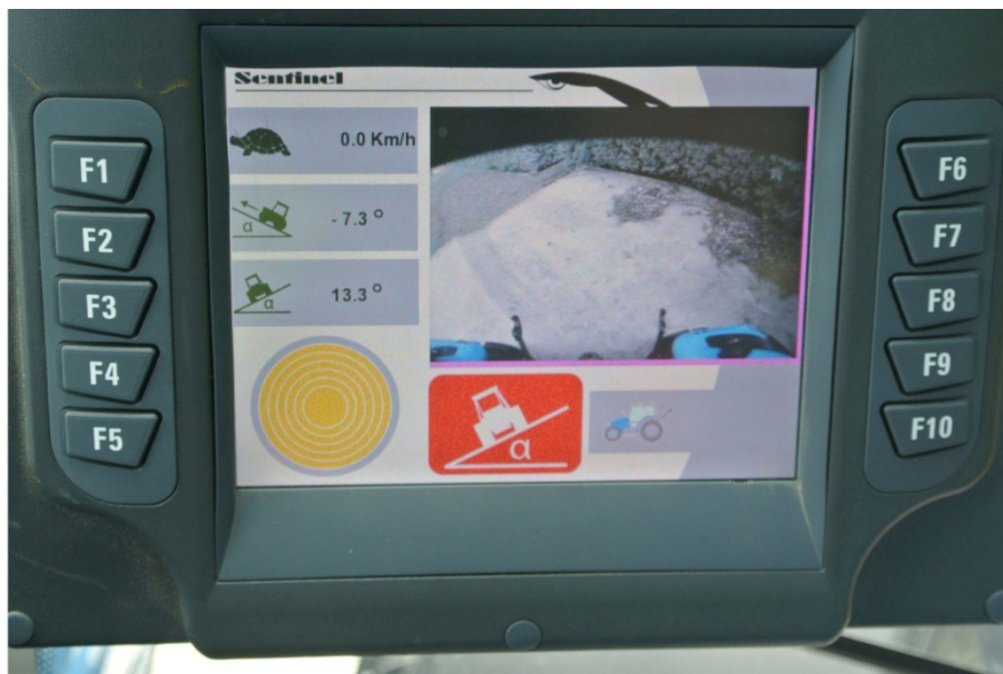
Figure 37. Display device during the static test.
