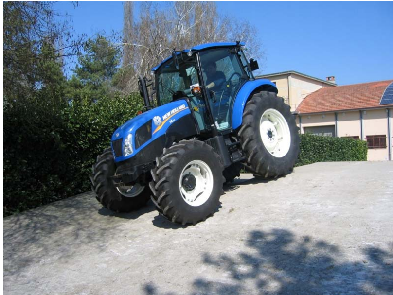
Figure 36. Tractor on the test slope during the static tests.
