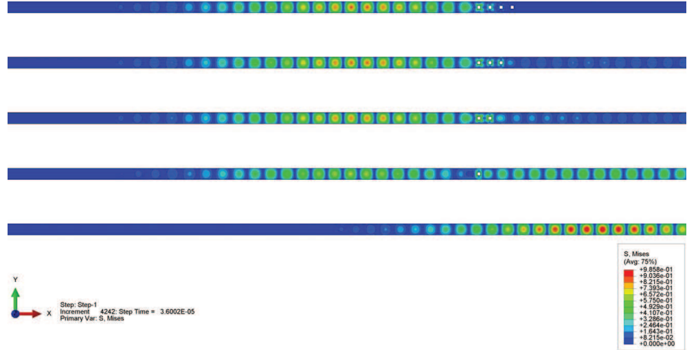
Figure 6.9: Von Mises stress field (snapshots at 36 \mu\text{s} ) for the waveguide presented in Fig. 6.5 consisting of a central portion containing the finite PC sandwiched between two homogeneous regions. From the bottom to the top the number of unit cells is increased from 0 to 4.
