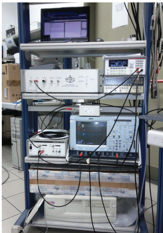
Figure 7.4: Measurement setup adopted in the PZT pitch-catch experiment to extract the transmission coefficient in the PVC phononic plate.
