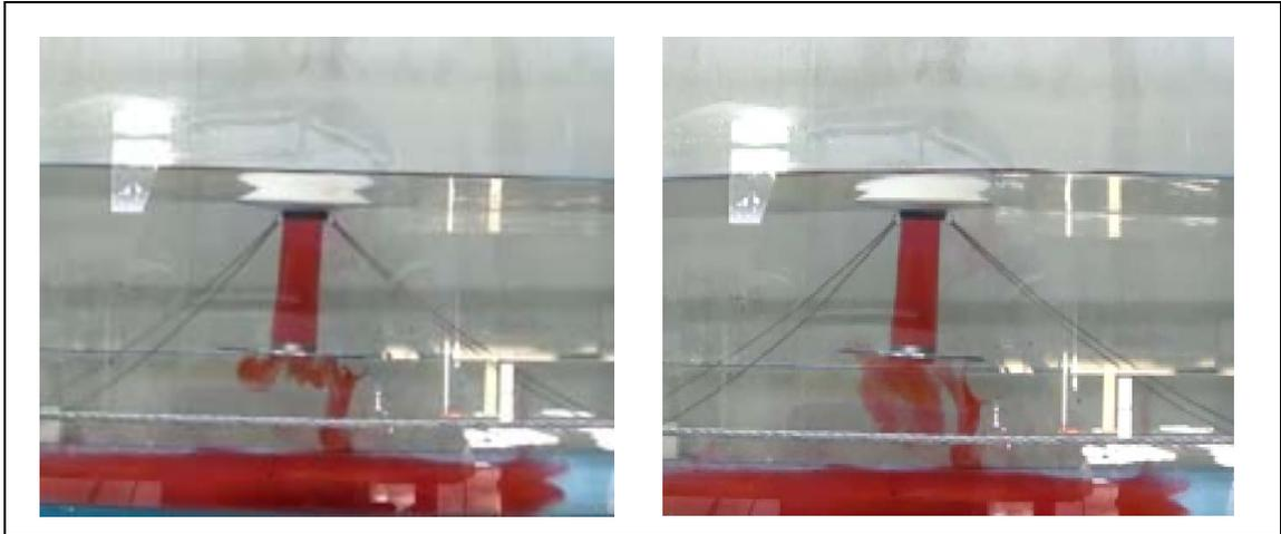
Figure 72: Eddy formation at the stabilizing ring, wave trough (left), wave crest (right)
