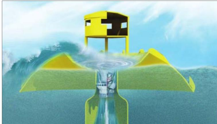
Figure 21: Spiral-reef overtopping wave energy converter, [83].
