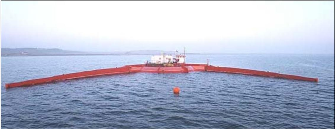
Figure 18: The Wave Dragon pilot plant (scale 1:4.5) in Nissum Bredning, Denmark, [89].
