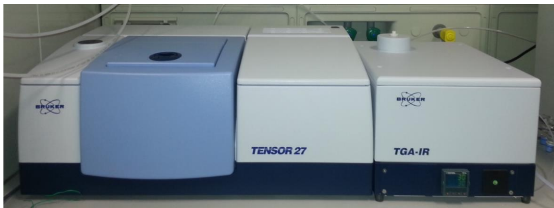
Figure 9.4 – FTIR spectrometer Bruker TENSOR 27 equipped with external gas cell.
