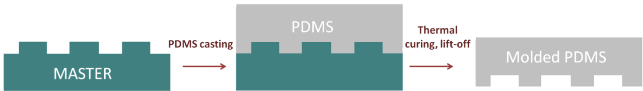
Figure 2- 3 Replica molding of the master with PDMS
