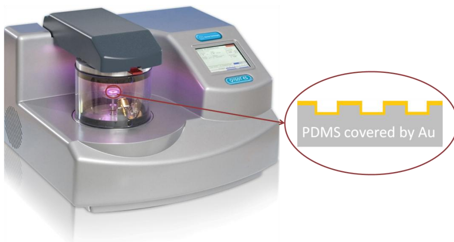
Figure 2- 4 Sputtering chamber under vacuum condition for Au deposition on PDMS
