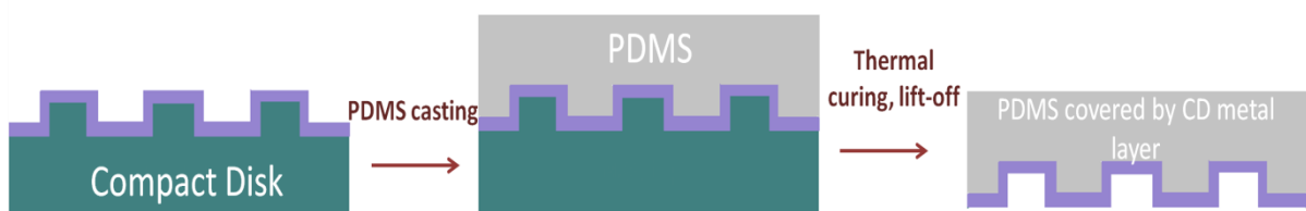
Figure 2- 5 Replica molding of the CD with PDMS
