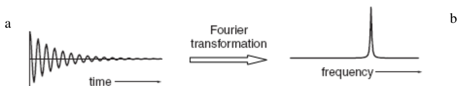
Figure 4. From FID (a) to spectrum (b) through FT transformation. Fourier transformation is the mathematical process which takes us from a function of time (the time domain), such as a FID, to a function of frequency, i. e. the spectrum.
