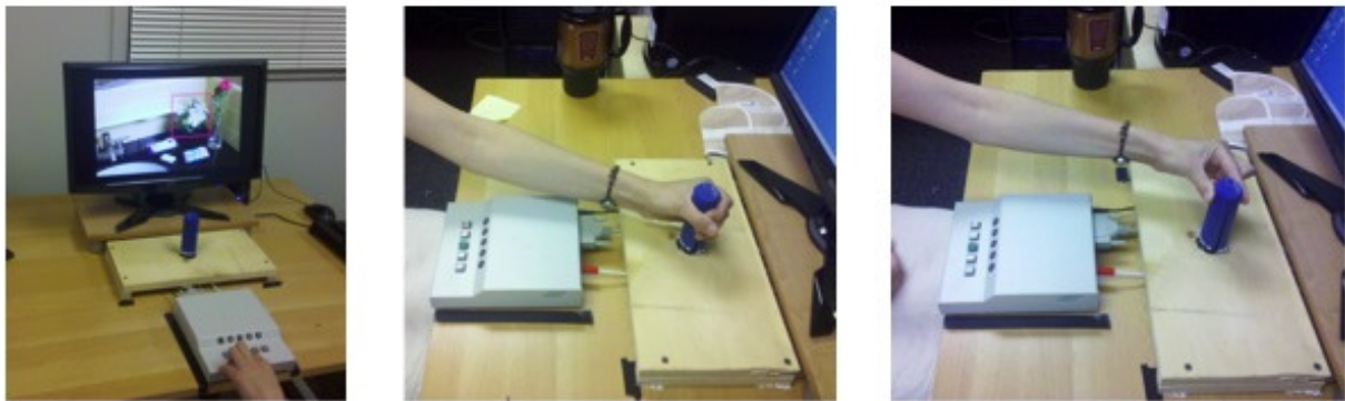
Figure 2. Experimental set up and use of the response device for clench and pinch grasps.
