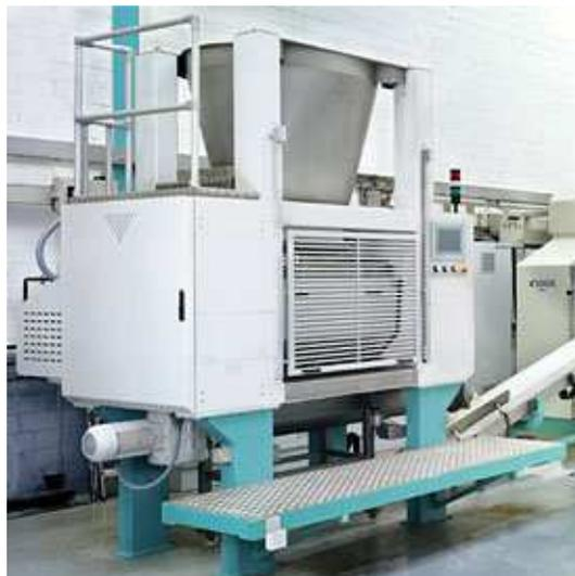
**Figure 6.** Pre-refiner machine equipped with three roller refiners (Buhler, 2013).
