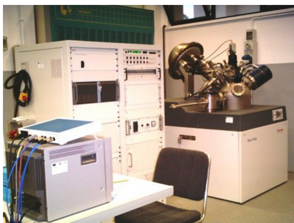
Figure 4.7.3. X-ray photoelectron spectroscopy system: XPS spectrometer and control unit.
