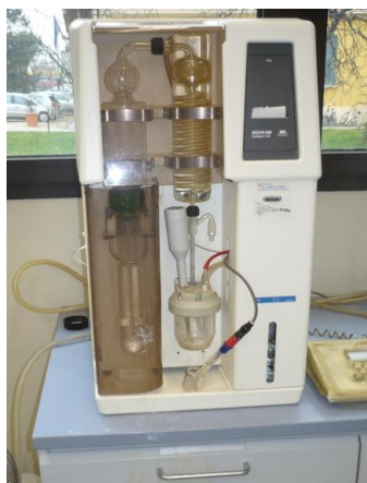
Figure 2.8. Büchi 339 unit used to distillate and titrate the sample for the total protein determination (Kjeldal).
