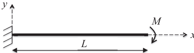
Figure 5.12: Cantilever beam under constant moment.
