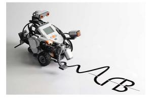
Figure 2.11: A differential wheeled mobile robot built with Lego Mindstorm NXT Kit.
