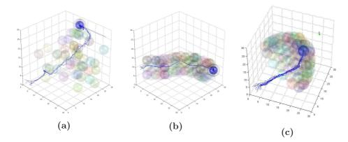
Figure 5.5: The presented technique is suitable to drive the AUV swarm in different scenarios, from the one with only dispersed obstacles to the heavily constrained one. The target can also be mobile (5.5a.).
