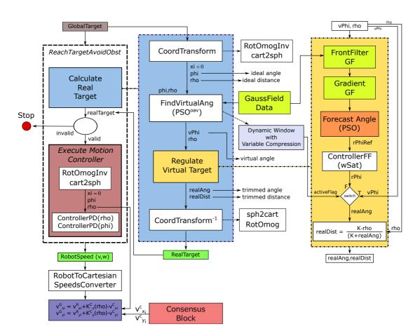
Figure 6.6: The global control scheme of the algorithm, from the robot's (agent's) point of view, is useful to better understand all the operations computed by the control system. Moreover it is possible to understand the interconnections between "classic" and modern control techniques as PSO and Consensus.
