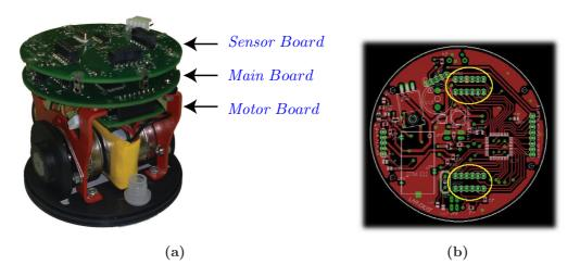
Figure 8.1: Prototype of the UniBot differential-wheeled mobile robot. In evidence the vertical bus on the main board's schema.
