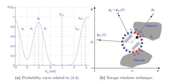
**Figure 4.3:** Example of escape window computed by considering obstacles detected by bumpers  $\{b_{17}, b_{18}, b_1\}$  and  $\{b_5, b_6, b_7\}$ .
