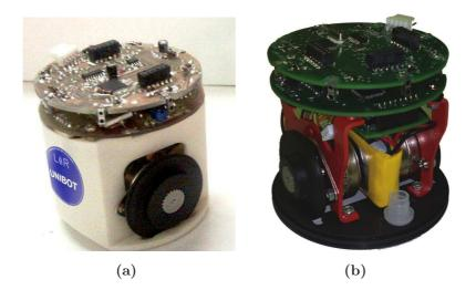
Figure 7.1: The prototype version (left) and the first full-functional version of Unibot  $V_1$  (right) have been the inspiration for designing the later version.
