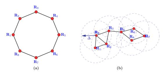
**Figure 3.4:** Examples of a 2D communication graph in case of  $||\mathcal{P}|| = 8$  with  $\Delta_i = \Delta$ ,  $i = 1 \dots 8$ : a *ring* graph, 3.4a, and a  $\Delta$ -disc graph, 3.4b.
