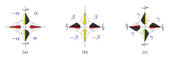
**Figure 5.2:** Rear view of the AUV with directional fins in  $\alpha, \beta, \gamma$  configurations.
