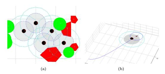
Figure 6.3: Obstacle detection is performed by sensors' device, providing the agent the possibility to perform obstacle avoidance while the agent is still computing the right control action to reach the final target. Notice that the sensor's area is clearly deformed by the presence of obstacles (6.3a).
