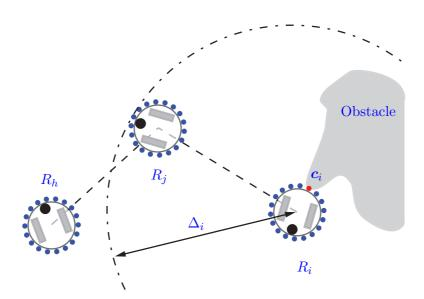
Figure 4.2: Example of broadcasted data for a collision. The dash-dotted circumference shows the communication area of robot  $R_i$  while dashed lines represent the inter-robot communication network.
