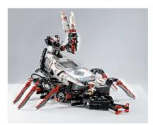
(g) An inverse pendulum disguised as a (h) A LEGO Mindstorms NXT- $EV_3$  scorbiped robot built with NXT- $EV_3$ . pion.
