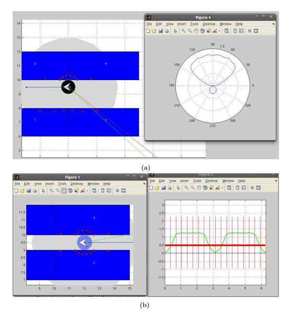
Figure 6.5: The Gaussian Field is used to detect obstacles and to perform obstacle avoidance. It is based on a Gaussian mask applied to the activated sensors when the robot encounters obstacles. The field can be represented as a continuous distance function on which the minimum values are calculated. The red line (visible in 6.5b), defined as the *valid threshold*, is the limit under which it is possible to consider the angle's aperture as free of collisions.
