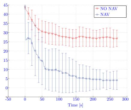
Figure 4.4: MSE and STDEV of distance error between each robot's position and the goal both with and without NAV. Data gathered over 20 simulations on Scenario 3.
