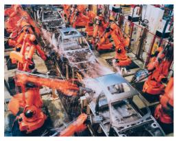
(a) An example of assembly-line where a chain of ABB robots produces automobiles.
