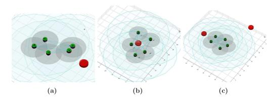
Figure 6.7: The soft formation control is performed by robots in order to avoid obstacles and remain connected.
