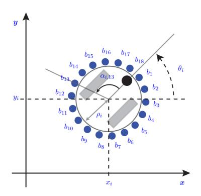
**Figure 4.1:** Kinematic model of the robots: the black dot identifies the robot's front,  $[b_1 - b_{18}]$  are the bumpers, and  $\alpha_{i,j}$  is the angle of the *j*-th bumper.
