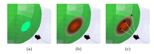
Figure 5.3: A circular collision area is produced when an AUV detects an obstacle (5.3a), such as the related virtual patch (5.3b) created as constraint, in the search space. Each virtual patch is defined by a 2D-Gaussian probability distribution that helps  $SA^{oav}$  in the computation of  $PSO^{oav}$ .
