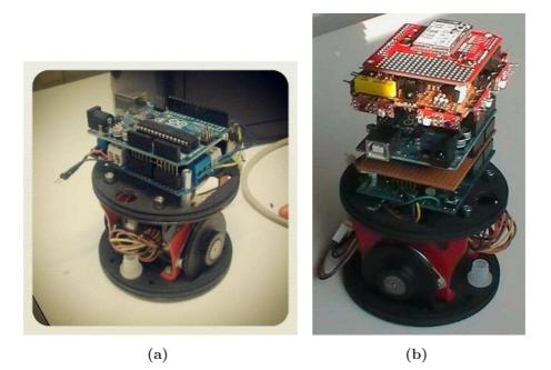
Figure 7.3: The A-Unibot prototype chassis with the main board (left) and the complete prototype equipped with a custom DIY square sensor board and the WiFy device.
