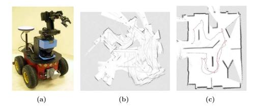
Figure 2.7: The 4 wheeled mobile platform Pioneer 3-AT, endowed with laser-scanner, GPS device, video-camera, robotic griper, ultrasonic sensors, is one of the best platforms used to study mobile robotics. By exploiting the laser scanner it is possible to build an environmental map (2.7b) which needs a post elaboration in order to be usefully exploited (2.7c).
