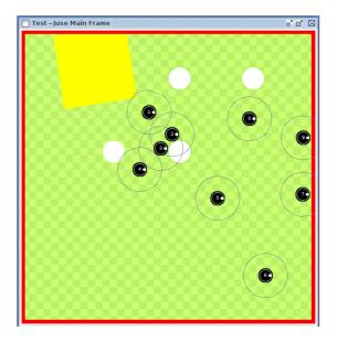
Figure 9.3: A top view of the simulated arena where a swarm of robots is performs a task. The depicted white circles are environmental obstacles, the yellow square a coloured area only. The obstacle detection performed by J.U.S.E. is based on the colours detected below the sensible area. This way it is quite simple to define if a coloured area is an obstacle or not.
