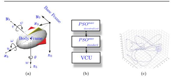
Figure 5.1: In order to define AUV's movements and to follow way-points, two different reference frames are needed, namely the Body and the Base Frame. By exploiting VCU's input variables, PSO control algorithm is able to change the AUV's attitude and speed, providing underwater navigation.
