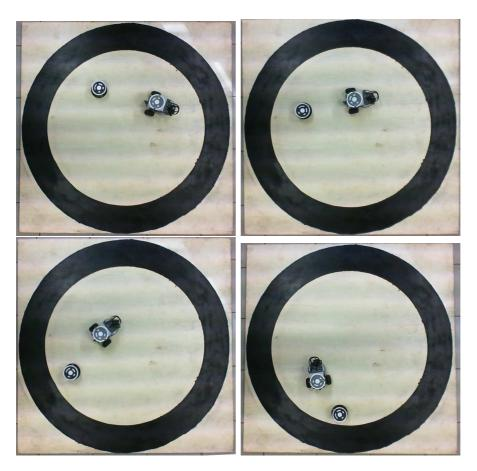
Figure 8.5: Snapshots of real experiments performed by students. The two robots, a UniBot and a Lego Mindstorm NXT, are engaged in a predator-prey algorithm. The black wide line around the arena, detected by the UniBot robot using its chromatic sensors, is used to delimit the escape area.
