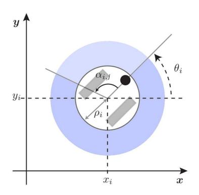
Figure 6.1: Kinematic model of the robots with the state variables. The blue ring represents the sensor's area defined by the 36 proximity sensors equally spaced around the robot, whose sensible distance and quantization can be freely configured. The parameter  $\alpha_{i,j}$  defines the angle of the  $j^{th}$  sensor.
