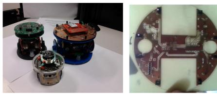
(a) A mobile robot comparison between (b) The future ground sensors' Unibot  $V_1$ ,  $V_2$  and E-puck.
