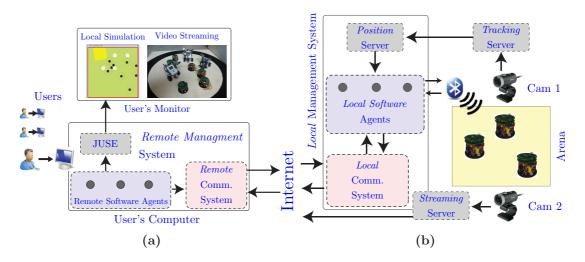
Figure 8.3: Scheme of the UniBot Remote Laboratory: Remote Management 8.3a and Local Management System 8.3b.
