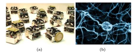
Figure 2.13: Alice (2.13a), developed at EPFL, is one of the most used mini-robots in the world. A very little area is large enough for the mobile robotics techniques applications that involve this robot model, because its dimensions are 2x2x2 cm. However the frontier of the robot dimensions' reduction process is in the nano-scale robotics. A futuristic vision of the nano-bots technology as substitution of neurons 2.13b may be representative of the future.
