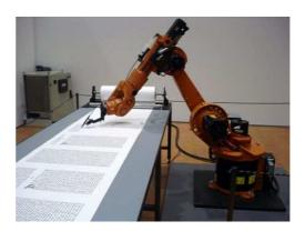
(b) A manlike-arm robot, produced by KUKA, is used as amanuensis.
