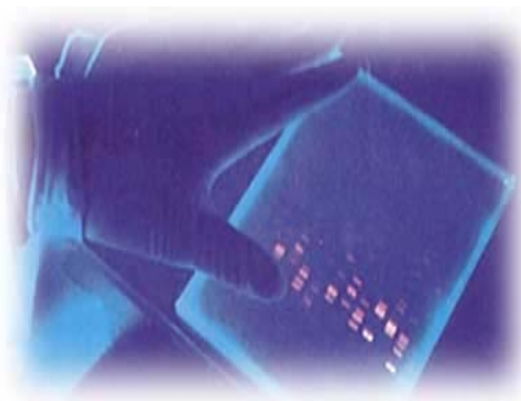
Figure 13. The DNA stained with ethidium bromide emits a red-orange fluorescence when subjected to UV light.
