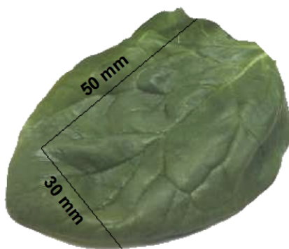
Figure 1. Sampling of tissues from spinach for calorimetric measurements. Sample size: height 50 \pm 1 mm, width 30 \pm 1 mm.
