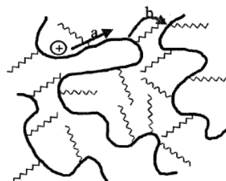
Figure 1.11: Schematization of the variable range hopping in an amorphous film of Pentacene.
