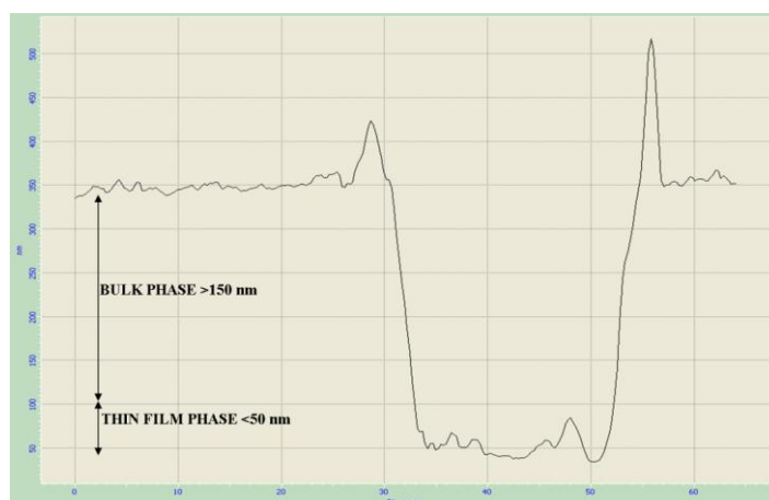
Figure 4.13: Profile of the edges of a scratch in a Pentacene layer 300 nm thick, measured by AFM in contact-mode. The separation in thin film phase and bulk phase is only appended to suggest the proportion of the two parts (75) .
