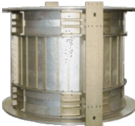
Figure 13 - The AMS-02 permanent magnet that operated [352] on board of the Space Shuttle Discovery in 1998 (Mission STS-91 - Experiment AMS-01).
