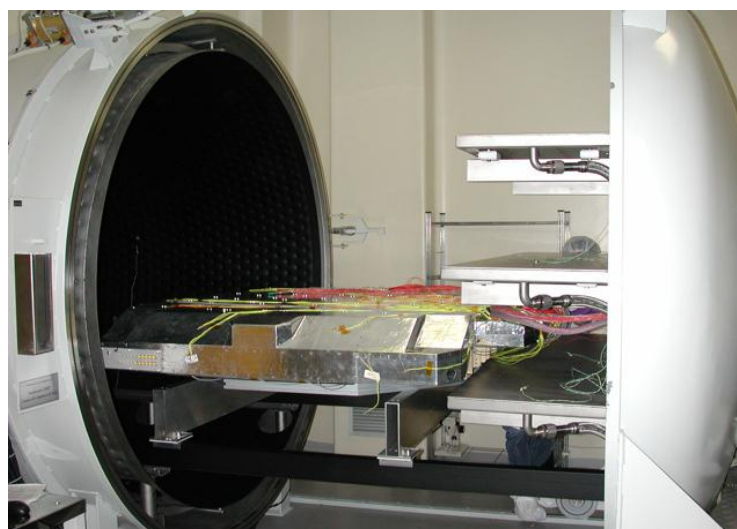
Figure 38 – The upper and lower TOF were located inside the vacuum chamber for the test.
