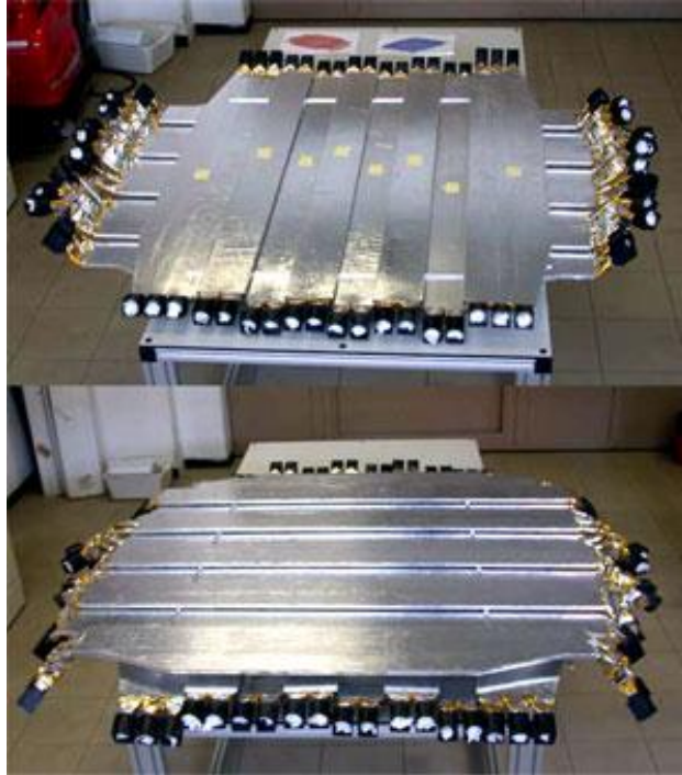
Figure 26 - The upper (a) and the lower (b) part of the TOF system. The PMT inclinations and directions are designed to minimize the effect of the magnetic field. The external detectors of each of the 4 floors of the TOF have trapezoidal shape, while the remaining 26 detectors have a rectangular shape. The two opposite ends of a counter are called p (positive with respect the TOF-AMS coordinate system) and n (negative) sides [388, 410].
