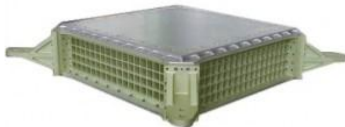
Figure 17 - The ECAL before the PMTs installation on the lateral slots (visible on the detector sides).
