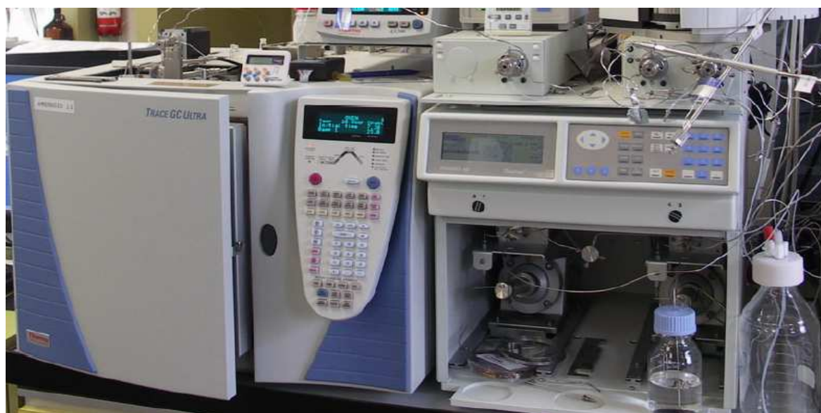
Figure 11. An example of LC-GC/FID system, consisting of a GC/FID instrument (left) equipped with an on line LC cleanup system (right).
