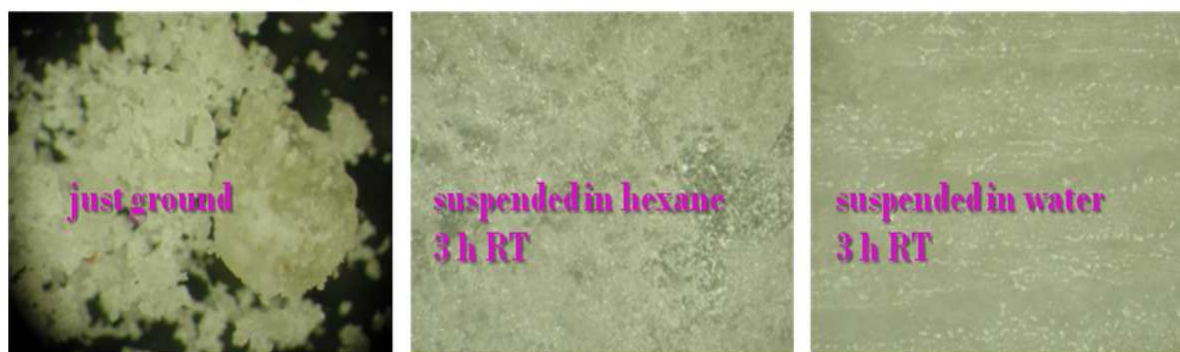
Figure 24. SEM images of handmade dry pasta after grounding (left), suspension in nonpolar solvent (middle) and in polar solvent (right). Hexane is not able to provoke food matrix swelling and opening. On the contrary, water allows to obtain a smooth food suspension.
