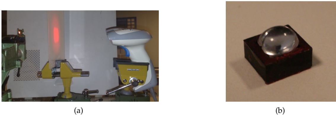
Figure 4.11: (a) Irradiance measurement set up. (b) Lens mounting on the LED .
