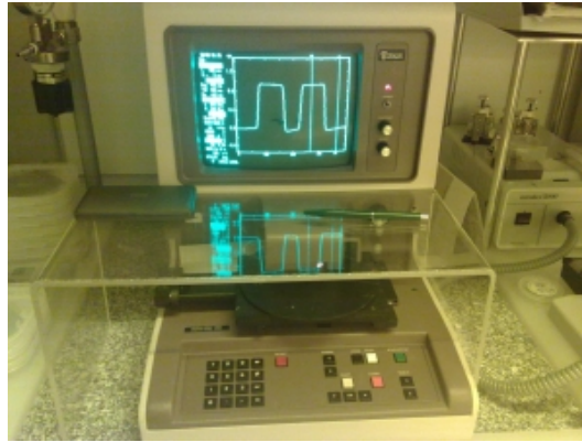
Figure 5.20: Machine for measuring the high level of the etching test samples.
