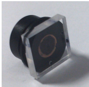
Figure 2.23: Phase mask sample glued to the lens barrel.
