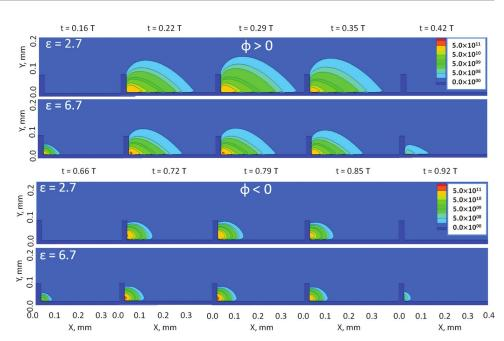
Figure 4.4: Discharge evolution for the positive (top) and the negative phase (bottom) compared for different values of  $\epsilon$ . The discharge area is shown at different time levels (T indicates the AC period).
