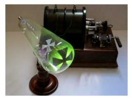
Figure 1.1: Crookes tube and power generation system.
