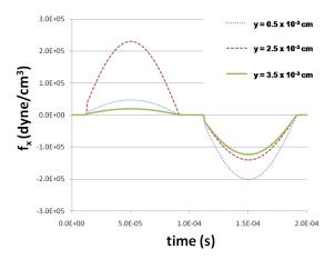
Figure 4.9: Sampled instantaneous x-force for different heights above the dielectric  $(6 \,\mu m \, \text{x-distance from the exposed electrode})$ .
