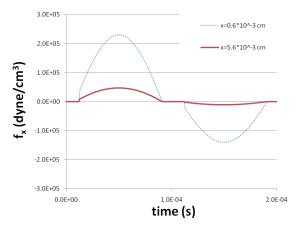
Figure 4.11: Sampled instantaneous x-force for different distances from the exposed electrode  $(y = 25 \,\mu m)$ .
