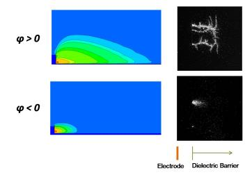
Figure 4.2: Drift-diffusion model validation: comparison between results and photos form above the dielectic surface.
