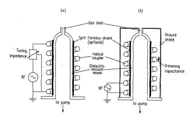
Figure 1.6: Cross sectional schematic diagrams of two inductively coupled plasma reactors: (a) helical coupler and (b) helical resonator [15].
