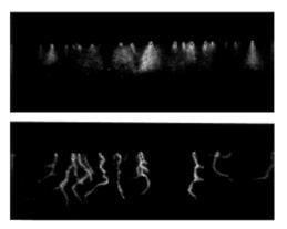
Figure 2.4: Difference between the negative (top) and positve (bottom) phase of DBD.
