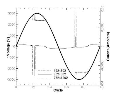
Figure 4.1: Dicharge voltage and total current over one AC period. Current unit is per cm depth in the z-direction
