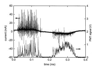
Figure 2.3: Current (top line) and light emission intensity (bottom line) during an AC cycle. The positive driven phase ranges form 0.0 to 0.2 ms and the negative one form 0.2 to 0.4 ms.
