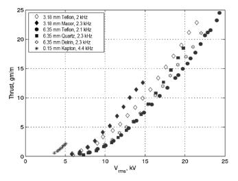
Figure 2.10: Thrust vs applied voltage for different dielectric materials. The thrust is measured by means of a force balance.
