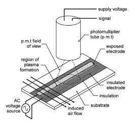
Figure 2.2: PMT setup for light emission measurements.
