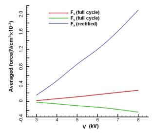
Figure 4.14: Time-Space averaged EHD force at different values of the applied voltage.
