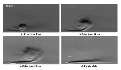
Figure 2.5: EHD starting transient, vortex visualization.
