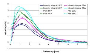
Figure 4.24: Comparison between velocity profiles (dashed line) and scaled intensity integrals (solid line) for four different power supply regimes at 30 mm form the upper electrode.
