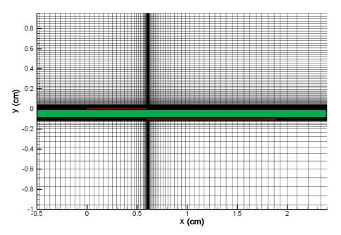
**Figure 3.4:** Computational domain with electrodes (red) and dielectric barrier (green).
