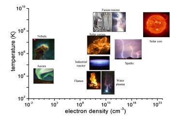
Figure 1.3: Plasmas varying in bulk gas temperature and electron number density.
