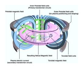
Figure 1.2: Magnetic plasma confinement developed for ITER.
