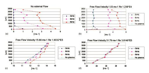
Figure 2.8: Induced flow motion for different values of AC frequency and free flow velocity.
