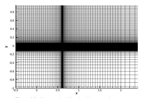
Figure 3.3: Computational domain with strong refinement near electrodes and dielectric surface.
