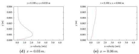
**Figure 4.17:** Simulated flow properties at t = 0.100 s. Velocity magnitude map (a) and temperature map (b). X-velocity line plots at different distancefrom the exposed electrode (c, d, e).
