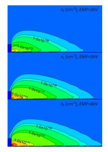
Figure 4.7: Discharge domain and ion concentration for different values of the applied voltage. In each case, pictures are taken for positive peak values of the applied voltage.
