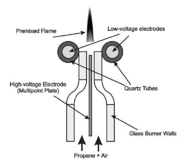
Figure 1.9: DBD apparatus for plasma assisted ignition.
