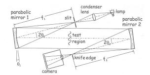
Figure 4.20: Z-configuration setup for Schlieren imaging.
