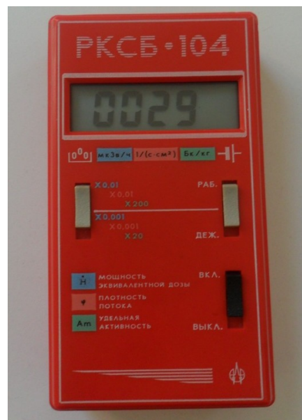
Fig.3.2 Photograph of PKCB-104 Geiger counter.
