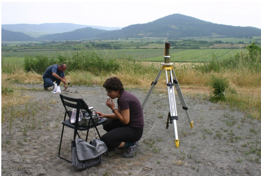
Fig. 3.12 Photograph of NaI detector placed one meter above the ground (sample V11).
