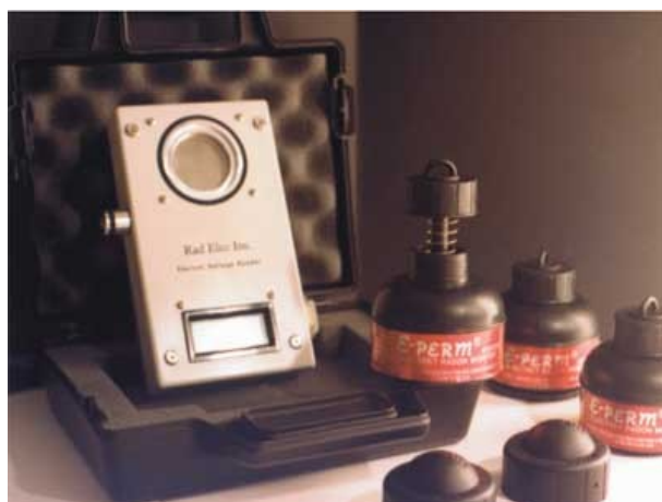
Fig.3.4 Photograph of E-Perm electret ion chambers opened and closed (on the right) and the electret reader (on the left).
