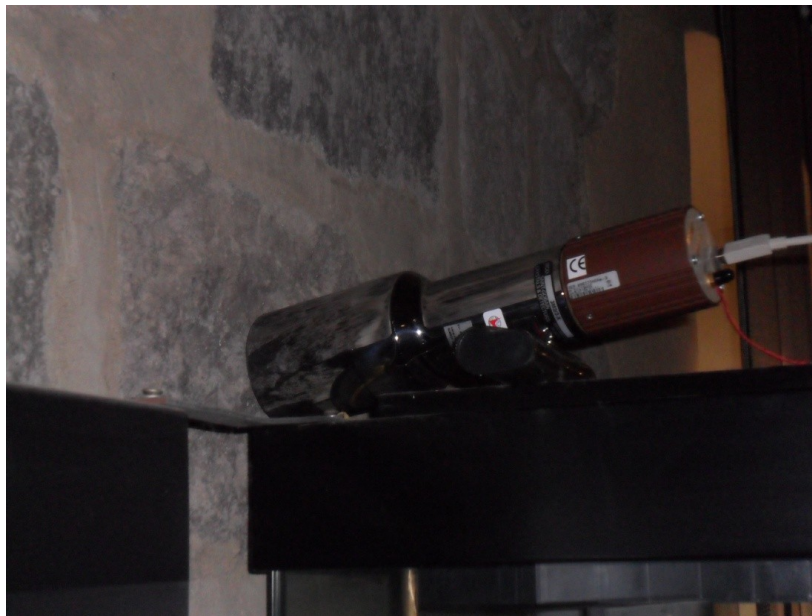
Fig. 3.19 Photograph of NaI detector used in indoor ambient, in the Fortress of Monaldeschi Cervara (on the top-left), particular of its external wall (on the top- right).
