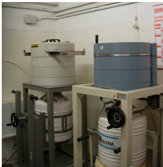
Fig. 3.9 Photograph of the two Germanium detectors (left-planar; right-coaxial) in the Laboratory of Environmental Radiochemistry of Bologna University
