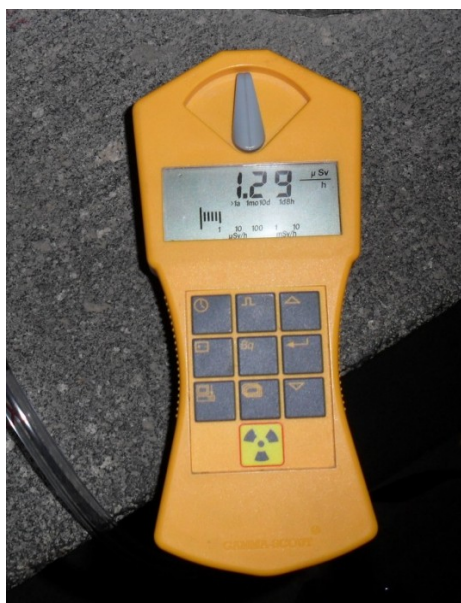
Fig.3.1 Photograph of Gamma-Scout Geiger counter.
